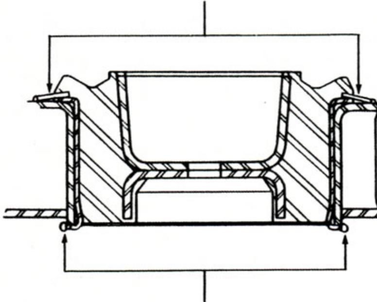
2. Bend retaining tabs outward and weld ends of tabs to crossmember.
