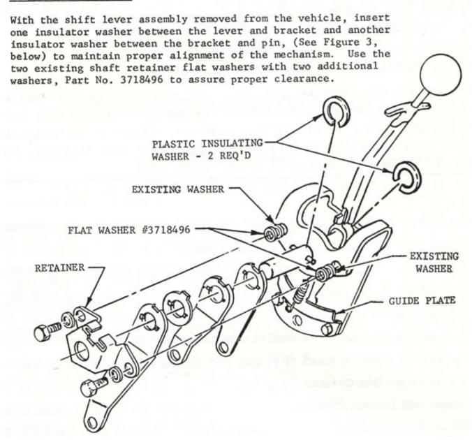
SHIFT LEVER TO GUIDE PLATE CLEARANCE
