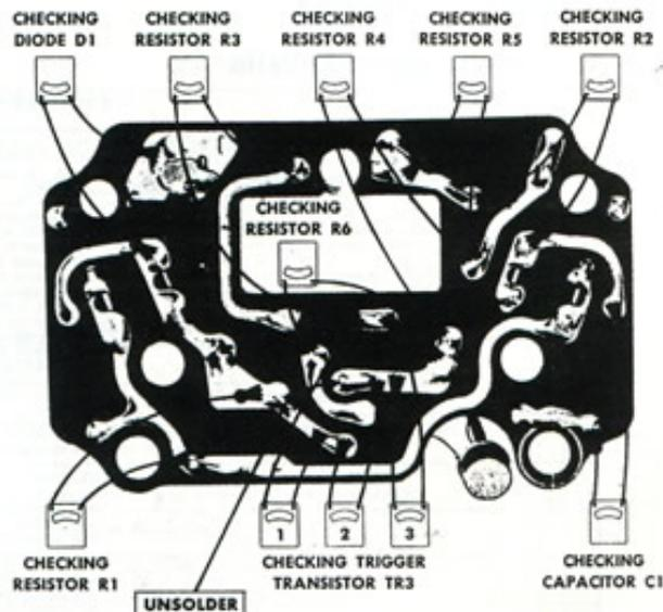
Figure 14—Checking component parts of amplifier shown in Figure 13.
