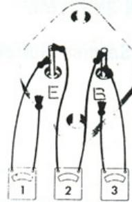
Figure 15—Checking Transistors TR-1 and TR-2.
