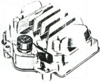
Figure 3—Typical ignition pulse amplifier.
