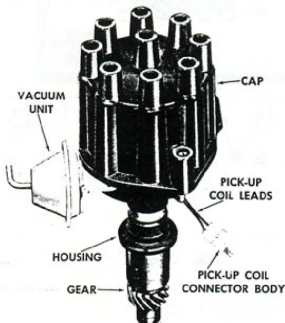
Figure 1—Typical magnetic pulse distributor.
