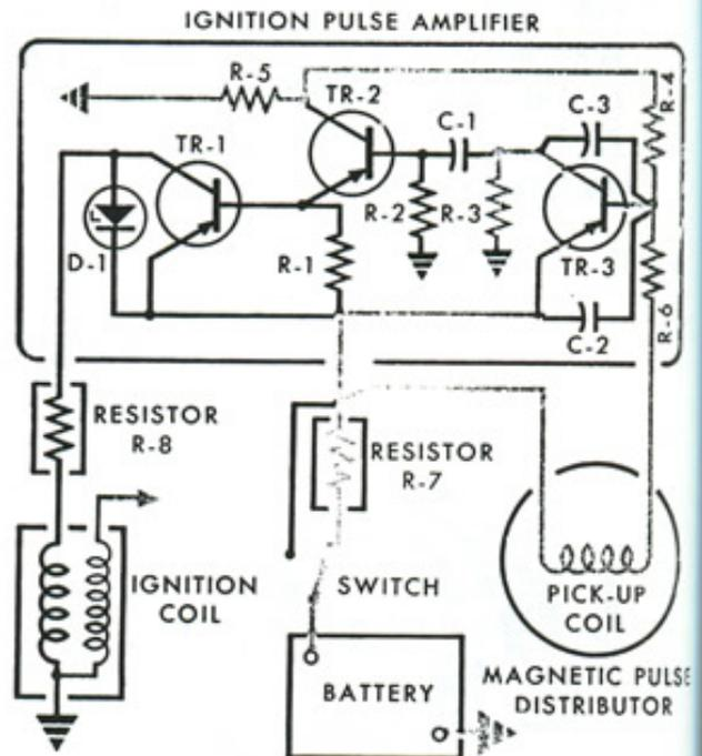
Figure 5—Internal wiring showing current flow in red with switch on and engine not running.
