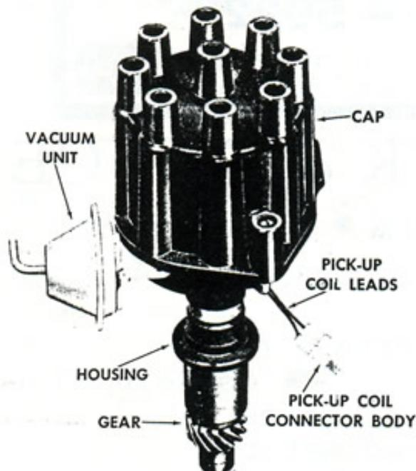
Figure 1—Typical magnetic pulse distributor.
