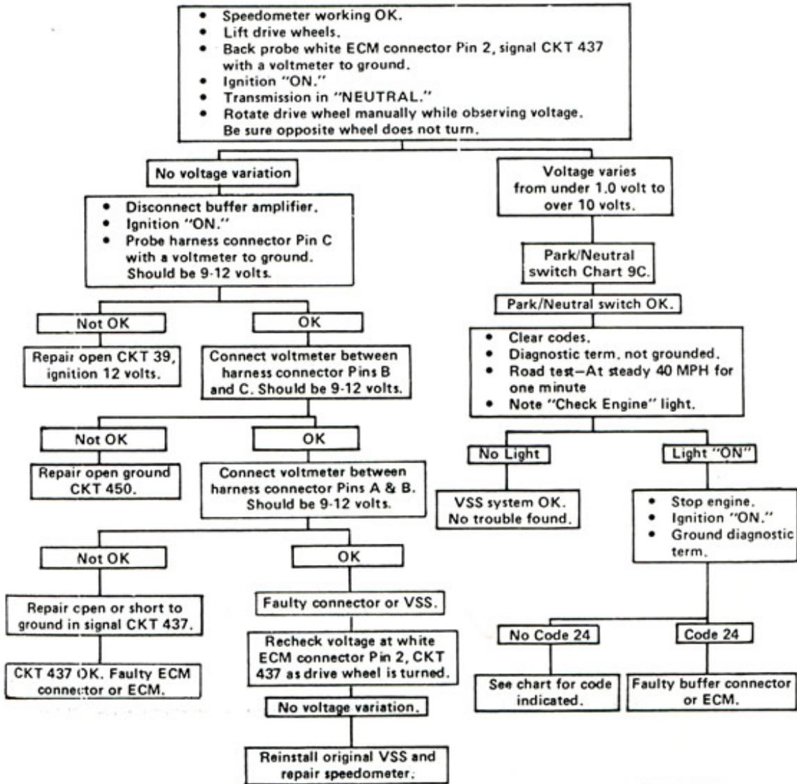
Clear codes and confirm "Closed Loop" operation and no "Check Engine" light.
