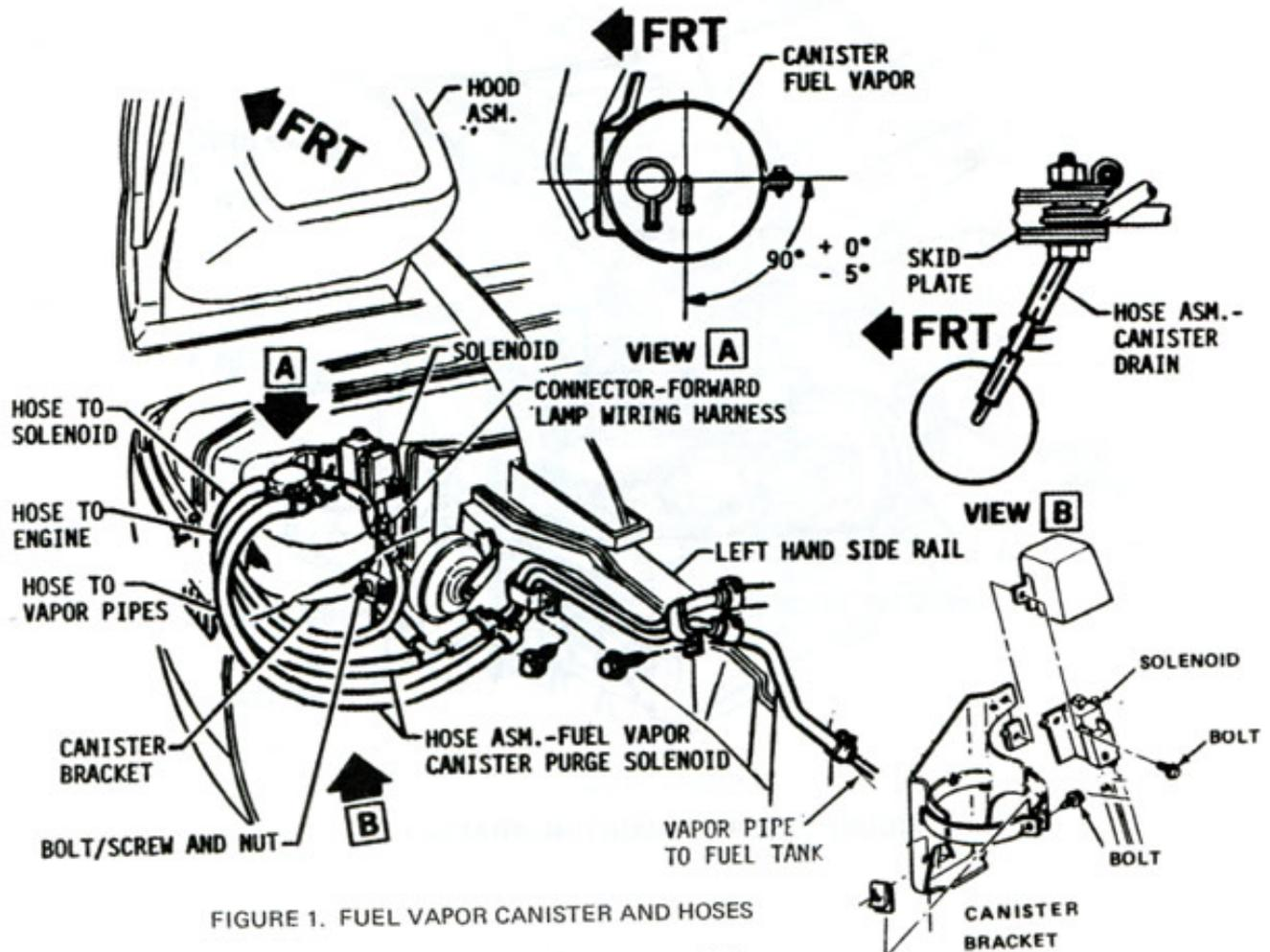
FIGURE 1. FUEL VAPOR CANISTER AND HOSES
