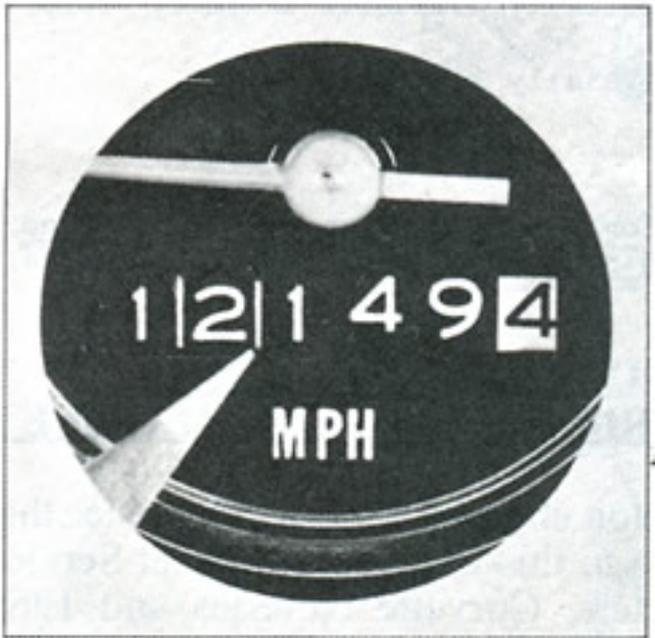
Fig. 40—Anti-Reversing Odometer
