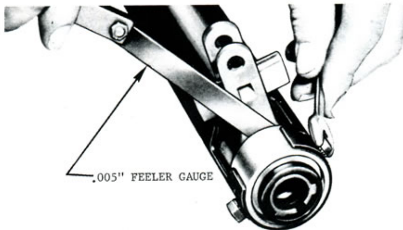
FIGURE 3 - ADJUSTING 1ST-REVERSE LEVER CLEARANCE
