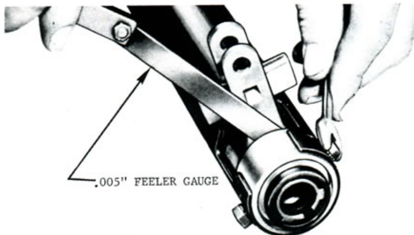
FIGURE 3 - ADJUSTING 1ST-REVERSE LEVER CLEARANCE
