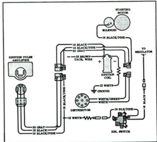
Fig. 5—Breakerless Ignition for Chevrolet Series 1000
