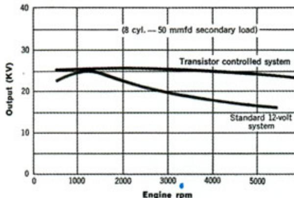
The accompanying chart of ignition system performance curves shows that the transistor controlled breakerless ignition system has greater output than the standard 12-volt system at all speeds, particularly at high speeds. While contact point deterioration problems limit primary current in the conventional system to about 4.5 amperes, the breakerless type could operate at as high as 7.0 amperes without damage to electric components.
