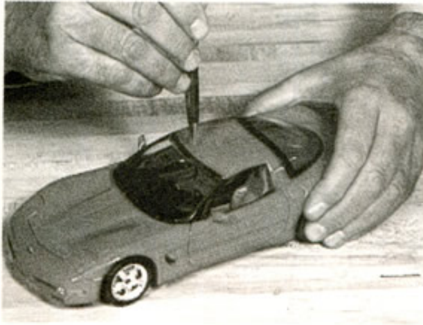
Pivot around vertical axis is called yaw.
