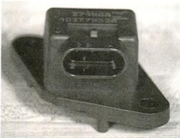
*Lateral accelerometer located beneath passenger seat*
