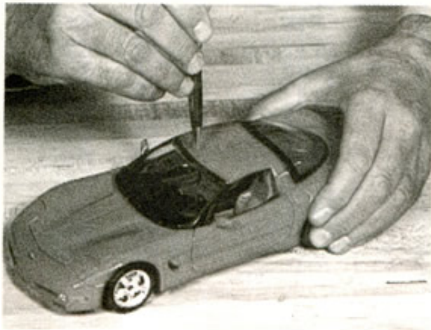
Pivot around vertical axis is called yaw.
