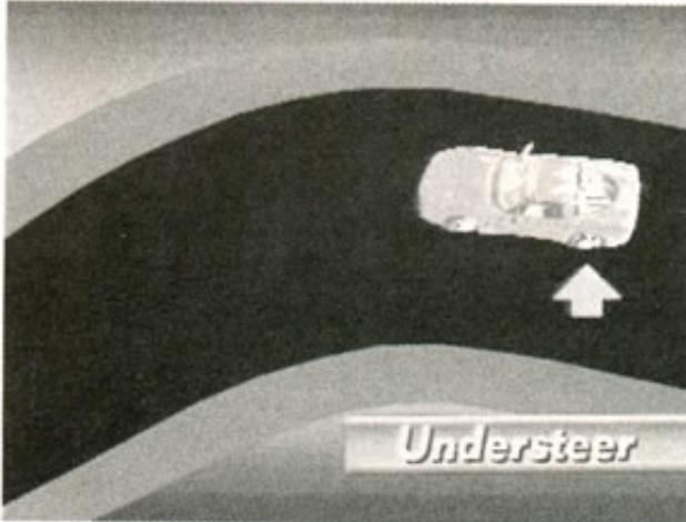
Active Handling system applies the inside rear brake to counteract understeer.
