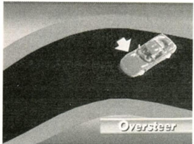
Active Handling system applies the outside front brake to counteract oversteer.
