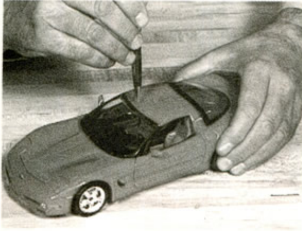
Pivot around vertical axis is called yaw.
