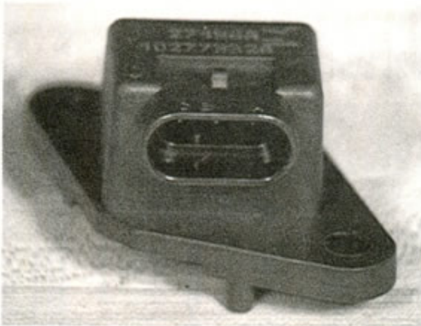
Lateral accelerometer located beneath passenger seat
