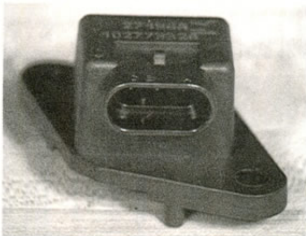
Lateral accelerometer located beneath passenger seat
