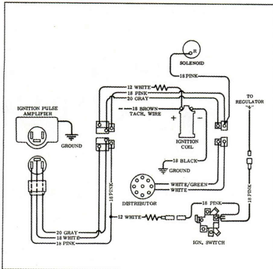
Fig. 6—Breakerless Ignition System—Chevrolet, Chevelle & Chevy II
