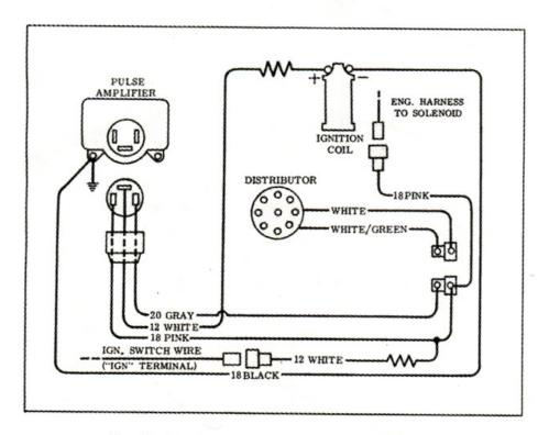
Fig. 7-Breakerless Ignition System-Corvette
