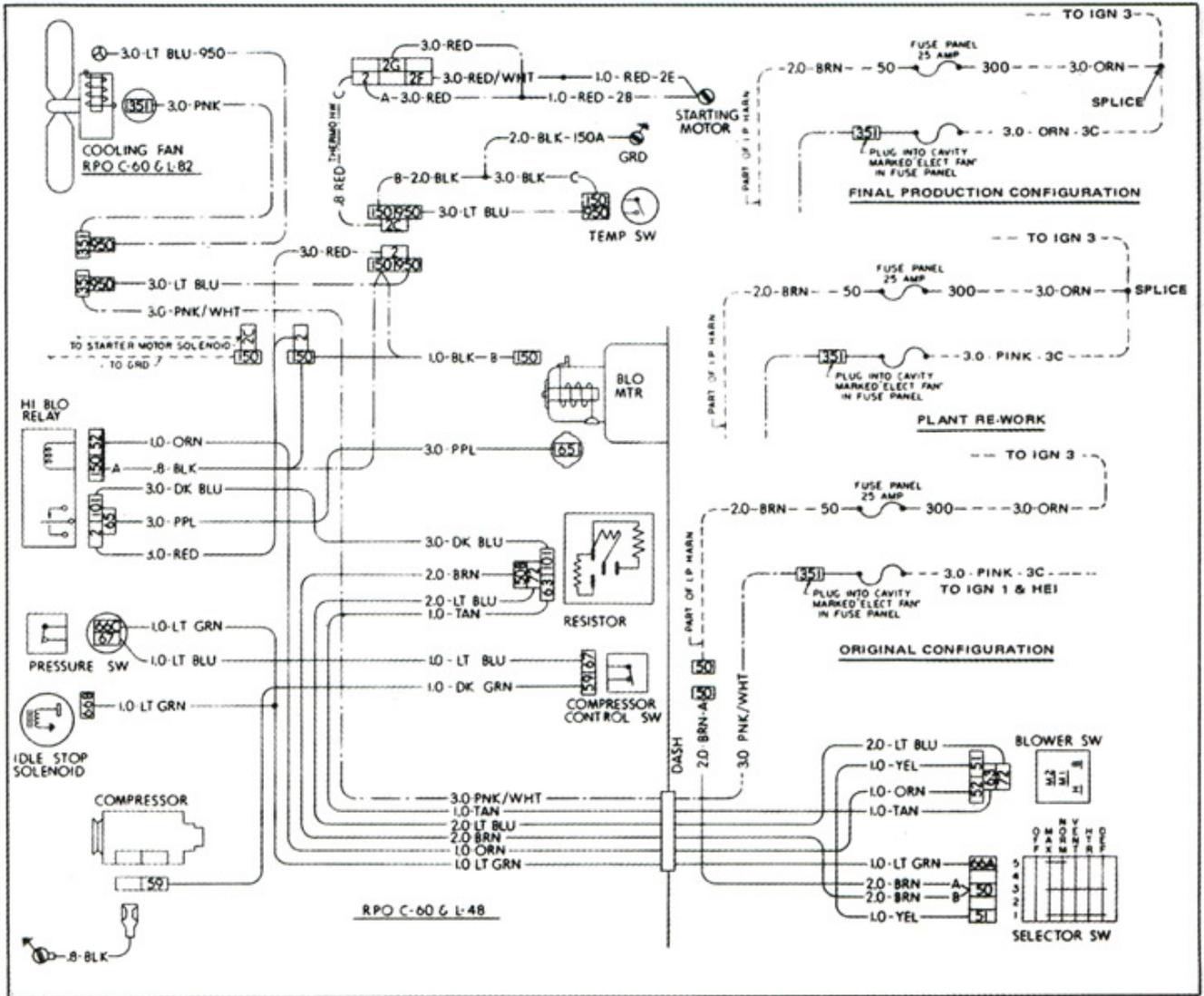
Fig. 4 — 1979 Corvette Auxiliary Cooling Fan Wiring Diagram
