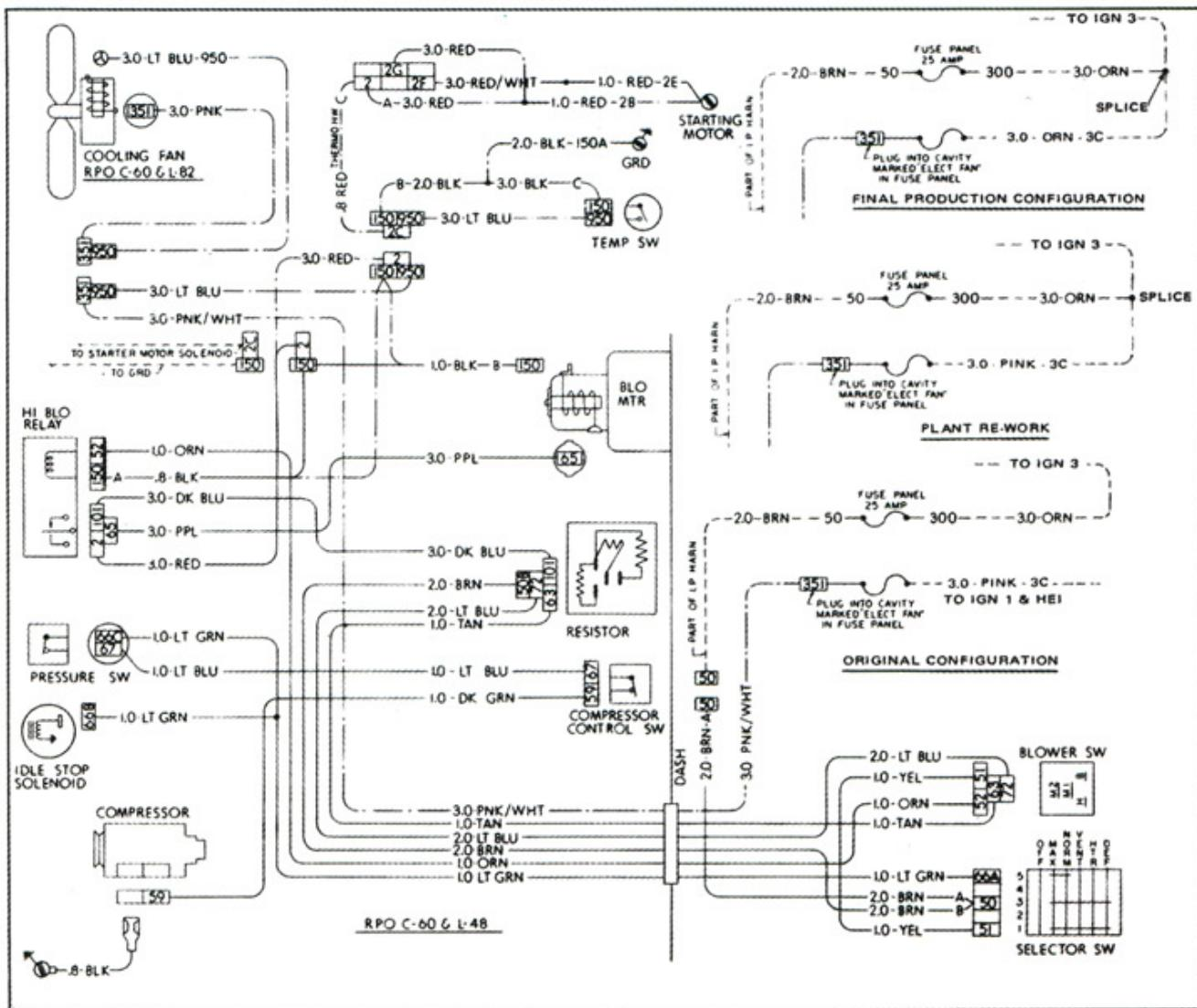
Fig. 4 — 1979 Corvette Auxiliary Cooling Fan Wiring Diagram
