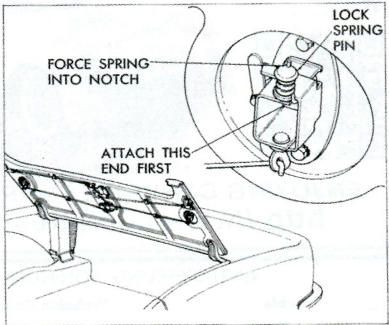
**Fig. 5—Corvette Bow Lock Spring**
