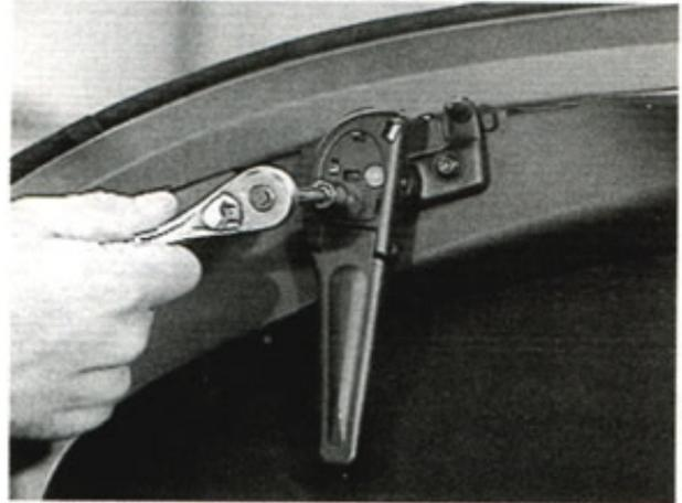
*Loosen two bolts on latch.*
