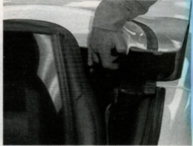
*Tonneau release located on underside of cover*
