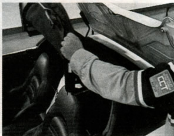
Top being raised from stowage compartment
