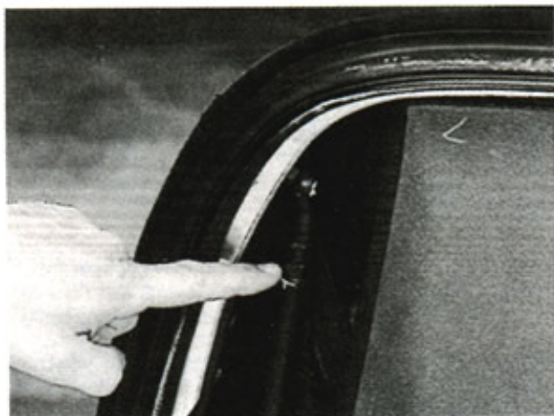
Adjustment screw for number 5 bow
