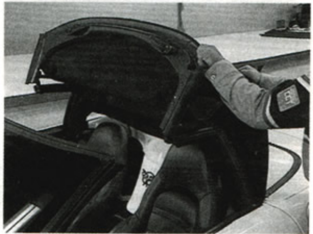
Numbers 1 and 5 bows in upward position
