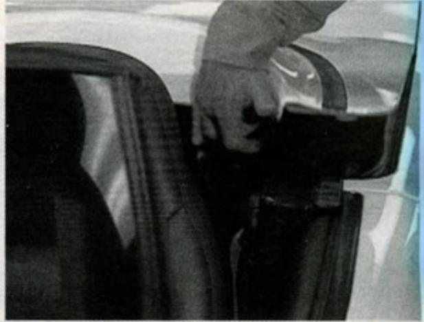
*Tonneau release located on underside of cover*
