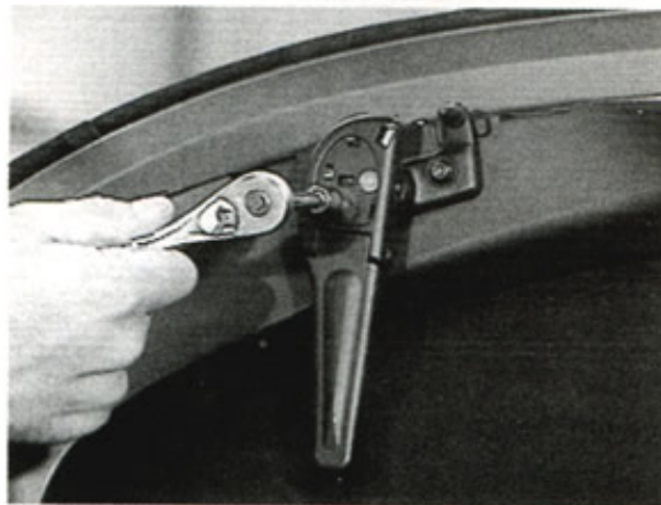
Loosen two bolts on latch.
