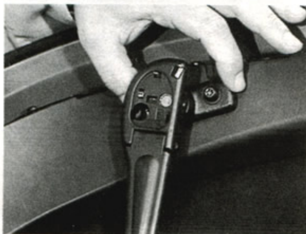
Adjust latch left or right.
