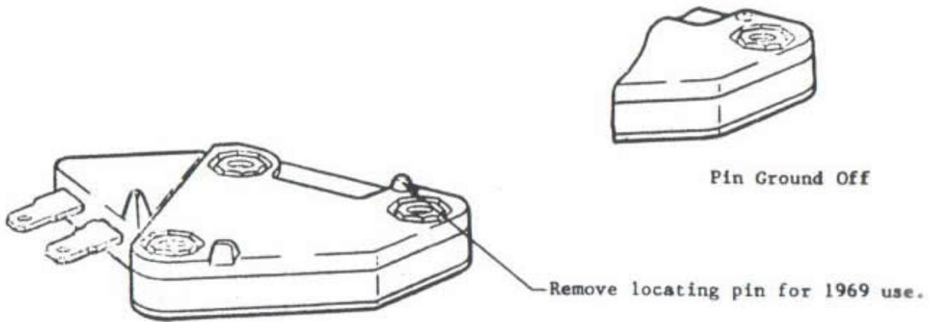
USING VOLTAGE REGULATOR IN 1969 DELCOTRONS
