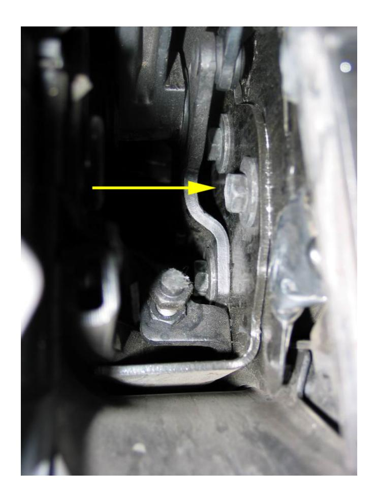
Now, the arrow is pointing to the 3 bolts, that are on each side that hold the top frame to the vehicle. I asked Ed to highlight these, because these 6 bolts are all that retain the top into the frame of the vehicle.
