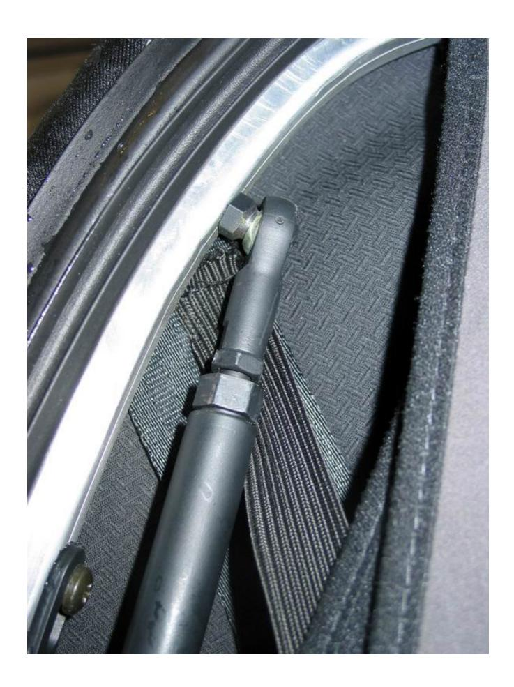
This is the close up for the adjustment on the #5 bow. Just remember, count the turns on the first side, and do the EXACT same thing on the other side. If you do not, you could bend the #5 bow. The 13 is your jamb nut, and the 15 is the actual adjustment.
