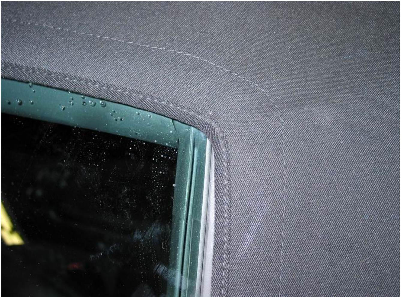
Just remember, that this adjustment will affect your tension on the latches on the windshield frame, and it should be known that you will have to put more effort on the top to latch it. This is due to the fact that you are changing the geometry of the top, and it is ok that it be this way. The tension will be lessened as time goes on.
