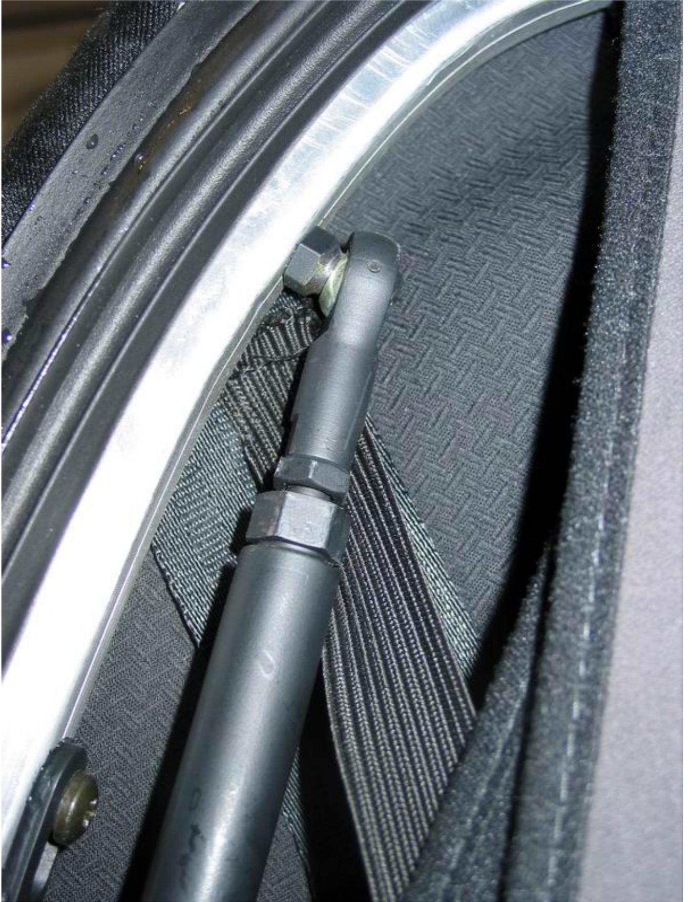
This is the close up for the adjustment on the #5 bow. Just remember, count the turns on the first side, and do the EXACT same thing on the other side. If you do not, you could bend the #5 bow. The 13 is your jamb nut, and the 15 is the actual adjustment.
