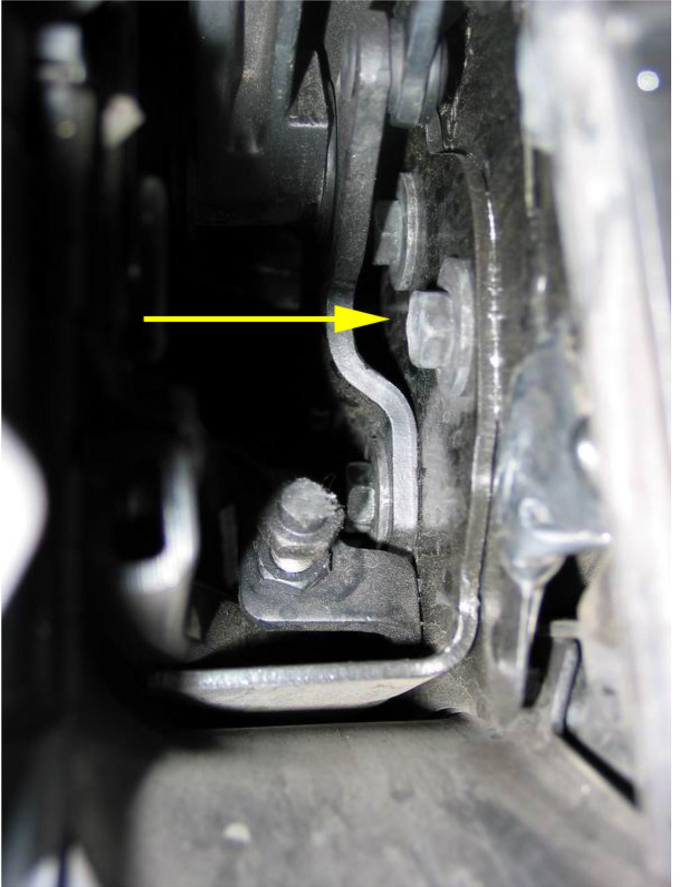
Now, the arrow is pointing to the 3 bolts, that are on each side that hold the top frame to the vehicle. I asked Ed to highlight these, because these 6 bolts are all that retain the top into the frame of the vehicle.
