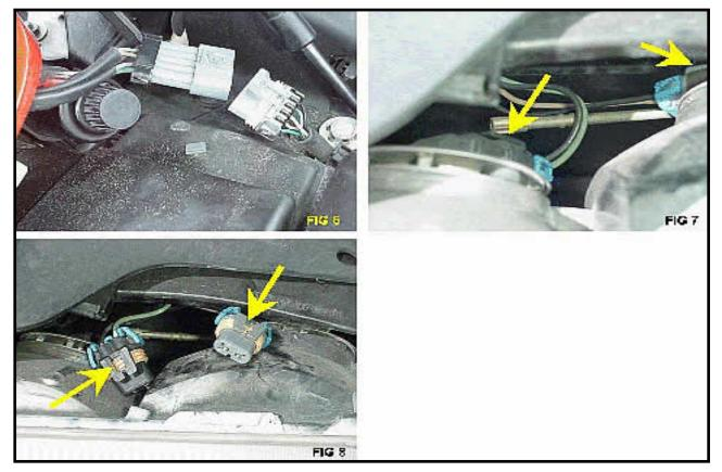
Now you can disconnect the main wiring harness (Fig. 6) and reach behind the lamps to disconnect those wiring harnesses (Figs. 7, 8). Be sure to note which one goes where. They are color coded.
