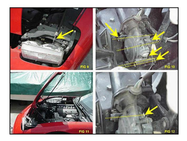
I used a bungee cord to support the headlamp assembly (Figs. 9 and 11 (my wife was too busy to help). The assembly will have nothing holding it up once the actuator is removed. I made sure that the bungee didn't put too much pressure on the unit. Just enough to hold it up.
