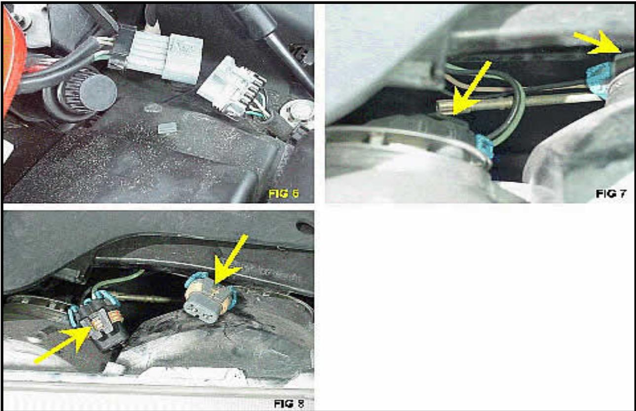
Now you can disconnect the main wiring harness (Fig. 6) and reach behind the lamps to disconnect those wiring harnesses (Figs. 7, 8). Be sure to note which one goes where. They are color coded.
