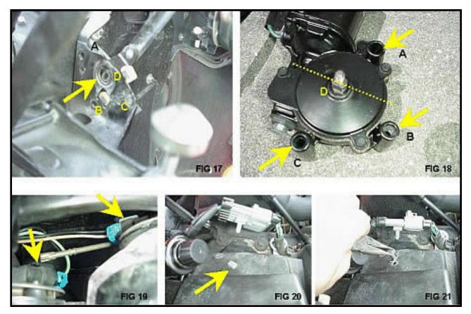
Figures 17 and 18 shows the four locations for the bolts and the shaft nut for the pivot arm.
