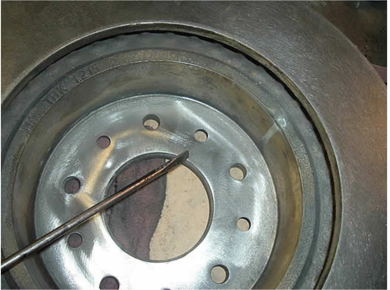
Notice the flat heads don't protrude beyond the tapped hole.
