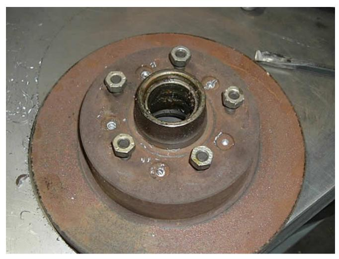
Here I have the rivets out and the rotor off. I drilled down just below the thickness of the rivet flange with a 5/16 bit. Then I use a cold chisel 90\* across the head to cut it in half.
