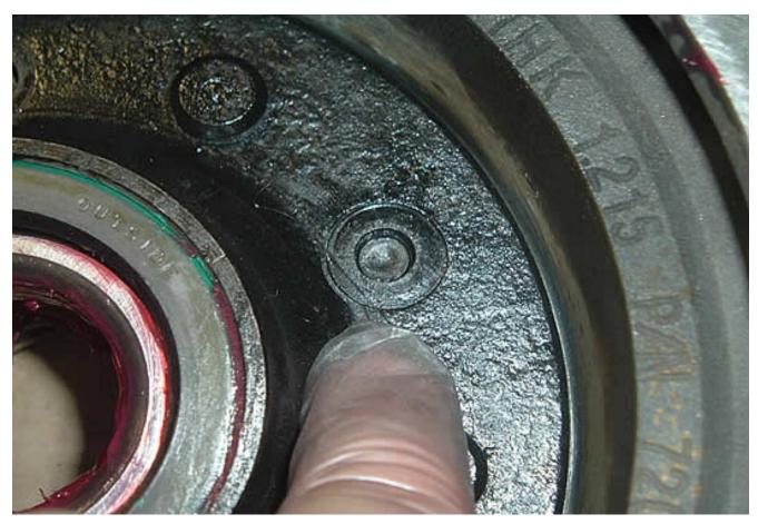
Here is the hub flange. Tapped 3/8-24 and the holes ground. Notice the turning lines still in the flange, there was no rust on this 35 year old part. The runout with the new rotor was .008" to start.
