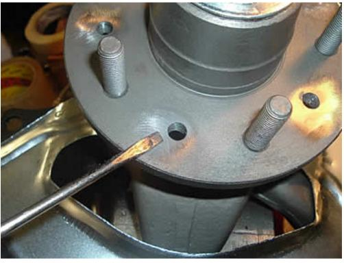
With the rotor bolted on and the bearings set to .001-.002 endplay I setup the indicator. I had to shim one location to get it just under .002" total runout. It's closer to .0015" but I marked it at .002'.
