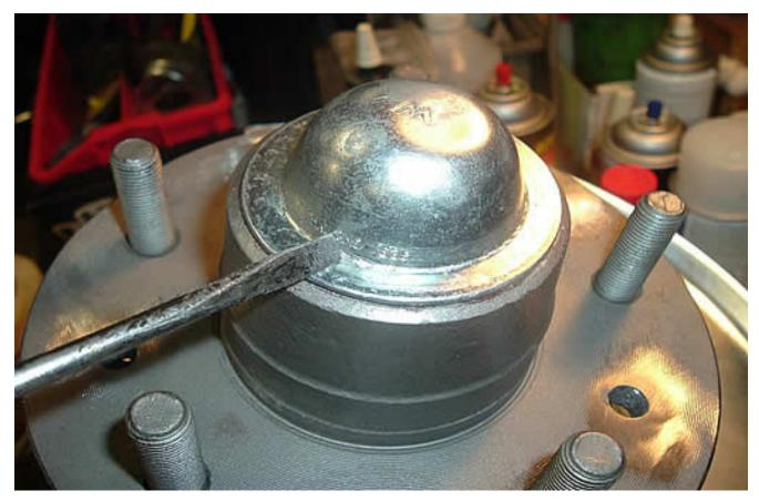
The cap's inner radius is tighter. I wondered why the bearings were getting snug after I set them up and installed the cap. The cotter pin was hitting the narrow inside angle and dragging. I installed a new pin and fit it under the cap with no drag.
