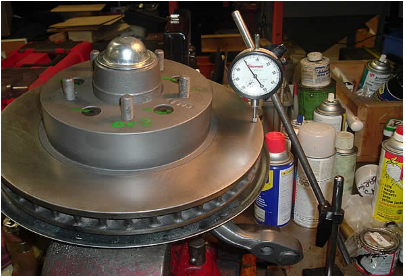
Here is the finished job. The green paint witness marks the rotor to hub location.
