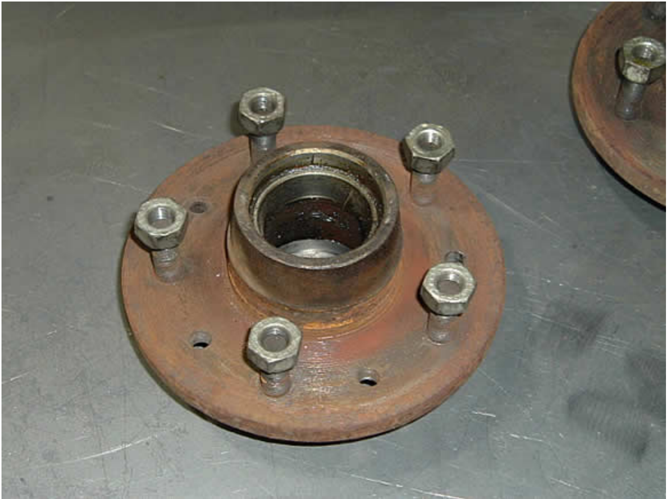
The rotor hat needs to be countersunk to use 3/8-24 socket flat heads.
