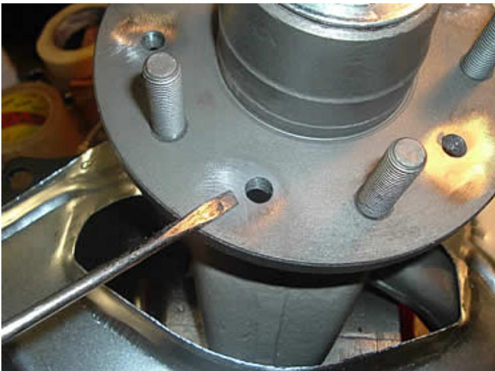
With the rotor bolted on and the bearings set to .001-.002 endplay I setup the indicator. I had to shim one location to get it just under .002" total runout. It's closer to .0015" but I marked it at .002'.
