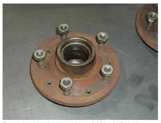
The rotor hat needs to be countersunk to use 3/8-24 socket flat heads.
