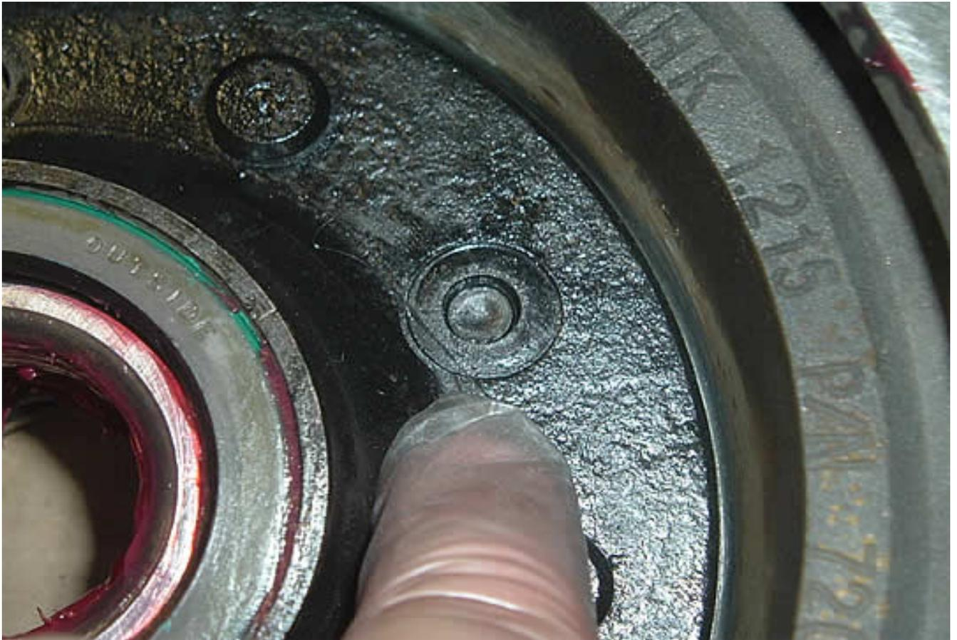
Here is the hub flange. Tapped 3/8-24 and the holes ground. Notice the turning lines still in the flange, there was no rust on this 35 year old part. The runout with the new rotor was .008" to start.
