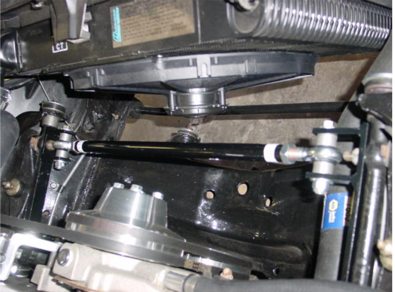
11. Adjust the spreader bar with just a touch of preload on it. When you get this done, tighten the jam nuts up against the spreader bar and you are done.
