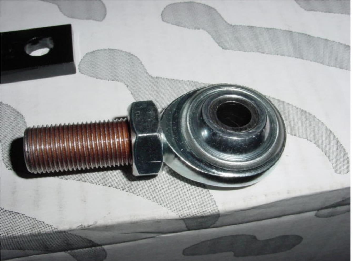
8. Place one end of the spreader bar between the ears of the spreader bar mount. Start the bolt through the mount, then put a bushing, then the heim joint, bushing and push the bolt through each part as you go. When you get the bolt completely through both ears of the mount, install a flat washer and the locknut.
