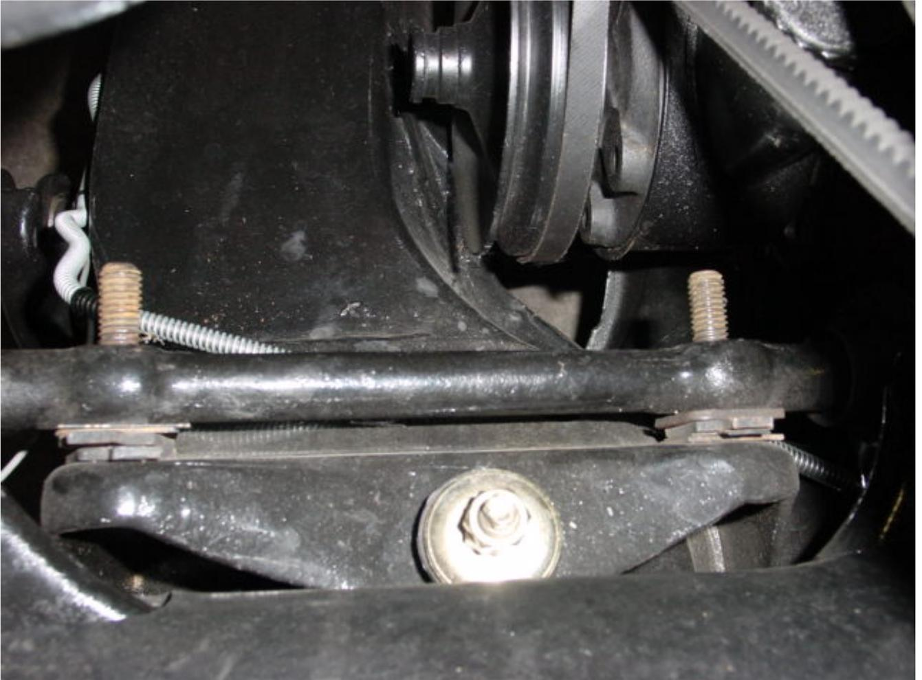
3. Remove both nuts on the upper cross shaft studs. Remove one about halfway at first, then start the second one and make sure your shims are gonna stay put. If they start to fall out, give the floor jack another pump.
