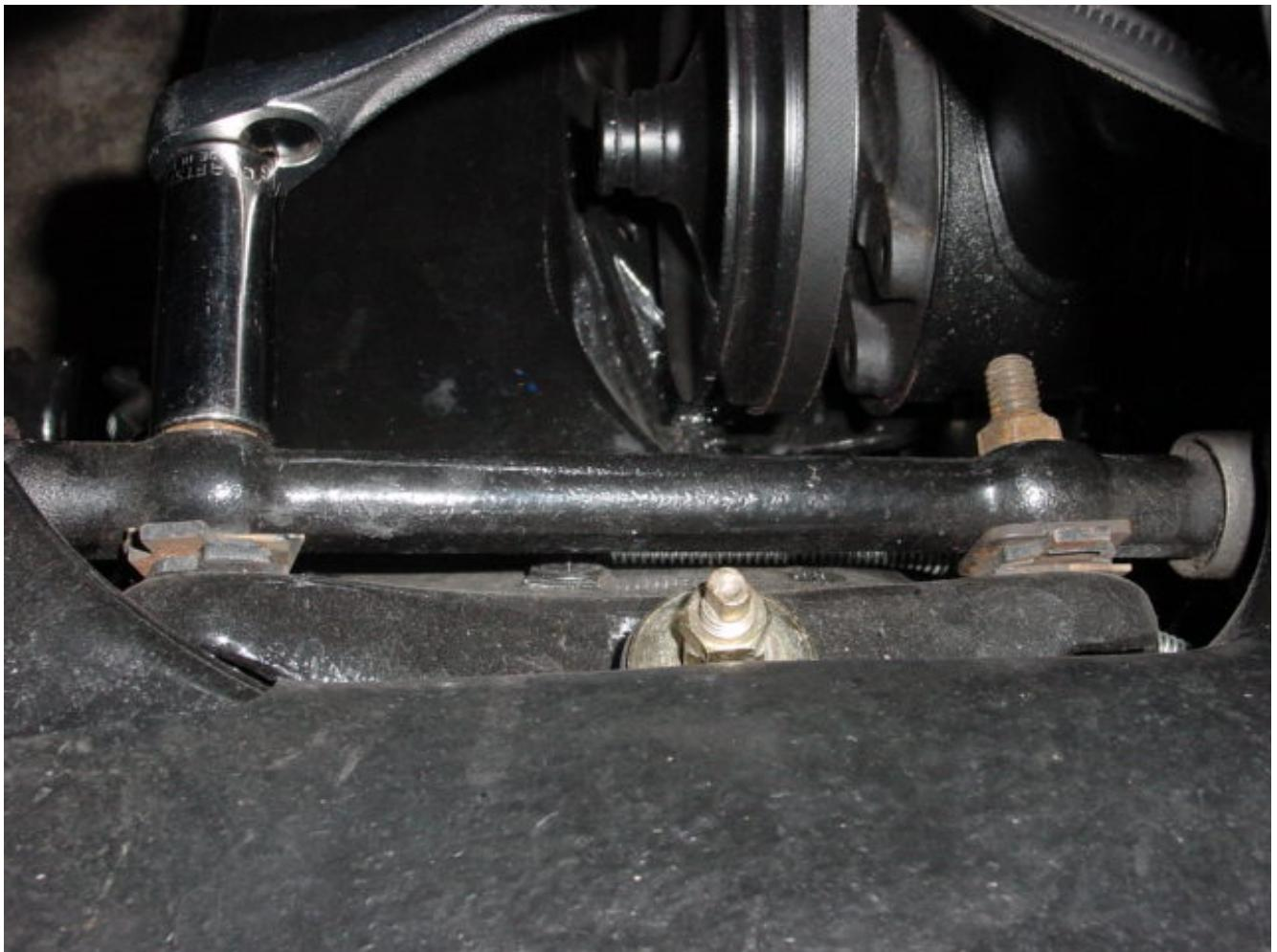
2. Put your floor jack under the frame rail just below the door. Lift the car just enough to take some weight off the front suspension. This will allow you to remove the nuts holding the upper a-arm cross shaft in place.
