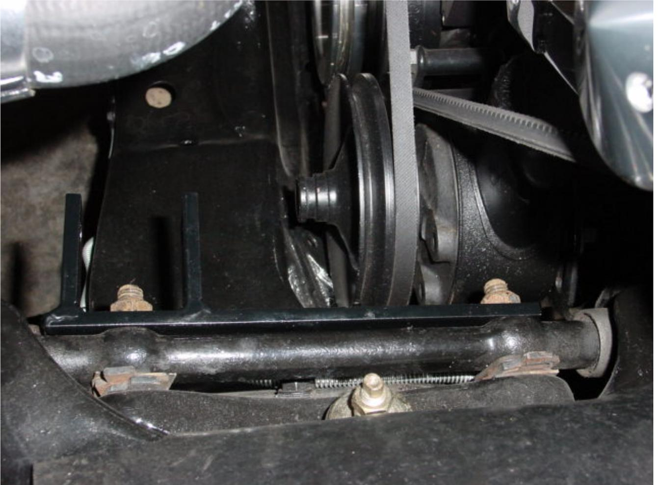
5. Ensure that all shims you counted are still in place as they should be and put the nuts back on. Let your car back down to the ground. See, that wasn't so hard.
