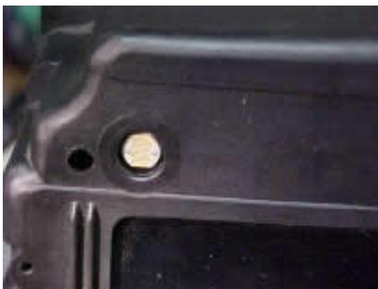
With the series resistor the cell will not sit all the way back in the hole in the front of the cluster. In this picture I used a  $\frac{1}{2}$  watt resistor (that's all I had). If you use a  $\frac{1}{4}$  watt resistor the photocell will be able to sit a little deeper in the hole.
