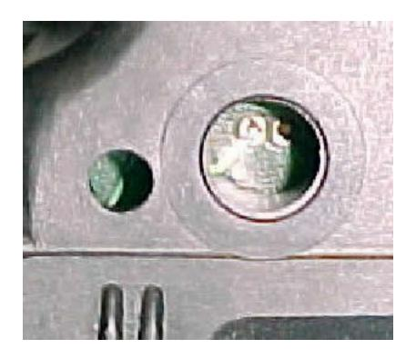
Once the old photocell is removed you will notice that the Radio Shack replacement is quite a bit larger than the old one. It will fit nicely in the hole in the cluster, you just won't use the plastic shroud that the old one did.
