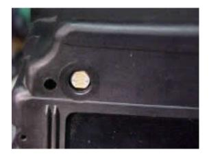
With the series resistor the cell will not sit all the way back in the hole in the front of the cluster. In this picture I used a ½ watt resistor (that's all I had). If you use a ¼ watt resistor the photocell will be able to sit a little deeper in the hole.
