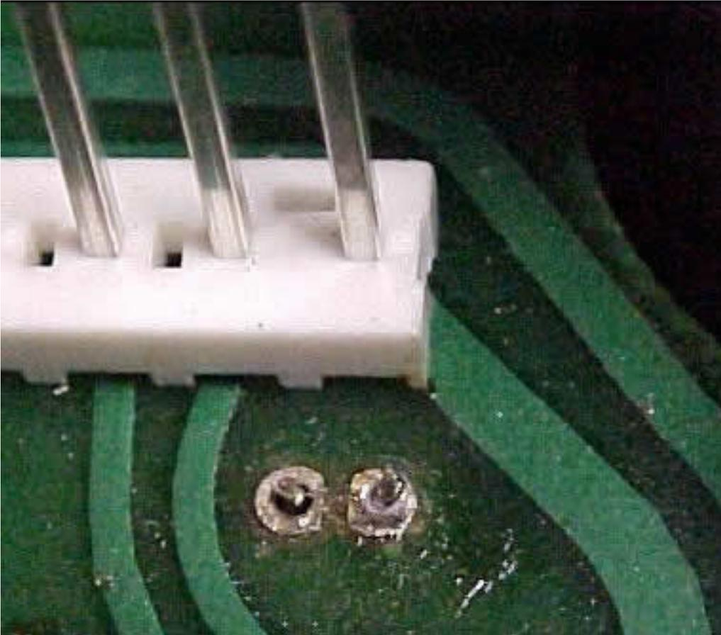
With a pair of tweezers you should be able to move the pin around inside the thru-hole in the board...that's when you know the solder has been removed. Be careful not to apply the heat of the soldering iron too long or the pad will lift off of the board, 5 seconds or so at a time should be enough.
