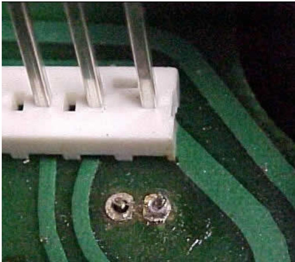
With a pair of tweezers you should be able to move the pin around inside the thru-hole in the board...that's when you know the solder has been removed. Be careful not to apply the heat of the soldering iron too long or the pad will lift off of the board, 5 seconds or so at a time should be enough.
