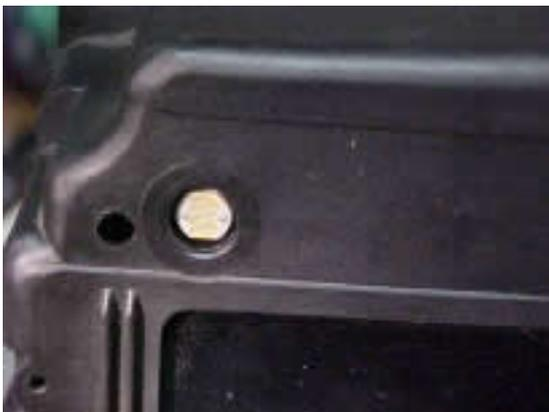
With the series resistor the cell will not sit all the way back in the hole in the front of the cluster. In this picture I used a  $\frac{1}{2}$  watt resistor (that's all I had). If you use a  $\frac{1}{4}$  watt resistor the photocell will be able to sit a little deeper in the hole.
