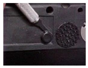
Using a good soldering iron and some solder wick, de-solder the old photocell and it can be pulled out of the front of the cluster (tip - put a little solder flux on the wick and it will work MUCH better).
