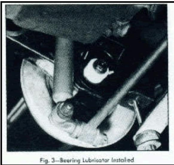
**Fig. 3—Bearing Lubricator Installed**
