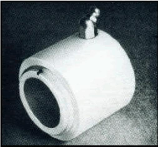
**Fig. 2 - Bearing Lubricator J-24488**
