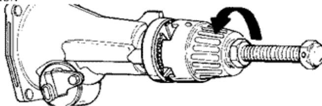
7. USE 15/16" WRENCH TO TURN BOLT CLOCKWISE AND REMOVE BUSHING
