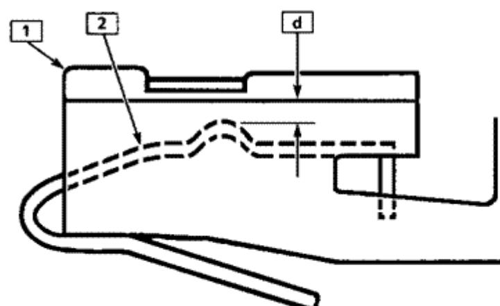
$d > 0$ , POOR TERMINAL CONTACT
