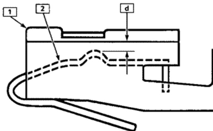
$d > 0$ , POOR TERMINAL CONTACT
