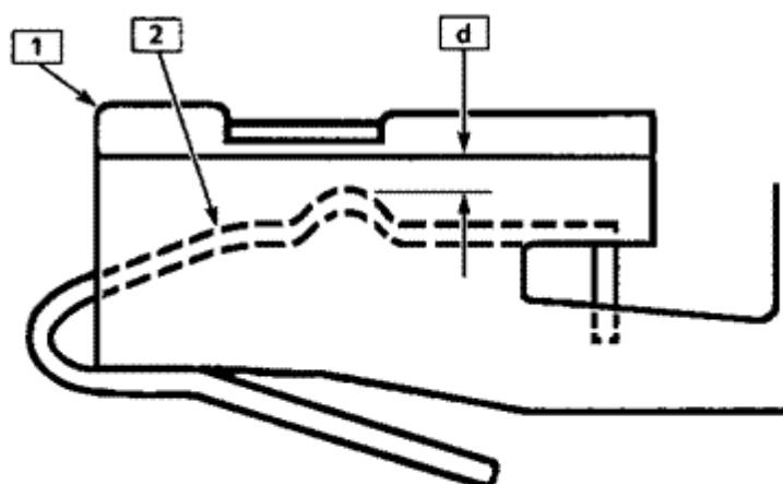
$d > 0$ , POOR TERMINAL CONTACT
