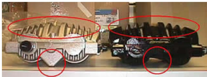
Main difference here is that the GS caliper is smoothed with the "CORVETTE" logo unlike the plain, ribbed J55 caliper.
