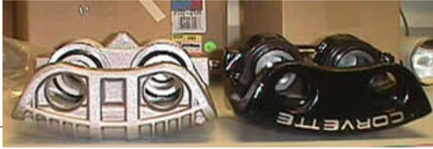
Another view of the top of the calipers showing the difference in ribs.
