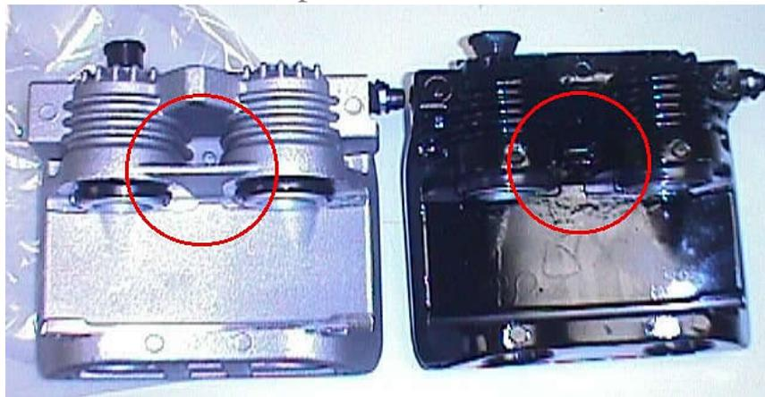
There are a couple of differences noticeable in this pic. First, the ribs on the top of the calipers. The J55 has more ribs but they are thinner than the ribs on the GS. Second, notice that the triangle shaped leg on the J55 caliper is not present on the GS.
