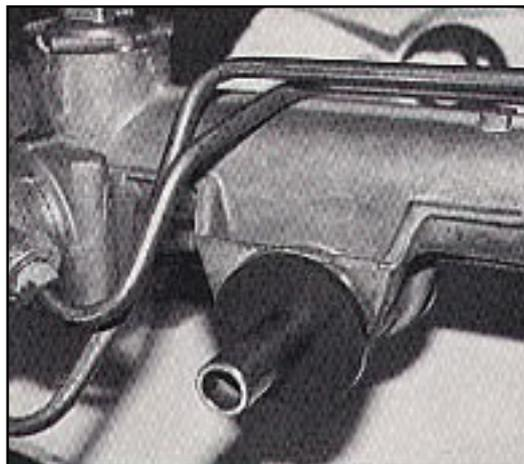
Install the inner tie rod dampener and boot and tighten the clamp. Then press out the left rubber and spacer and mount. Slide in the new polyurethane mounts and the new spacer. Then reinstall the steering rack in reverse order of disassembly.
