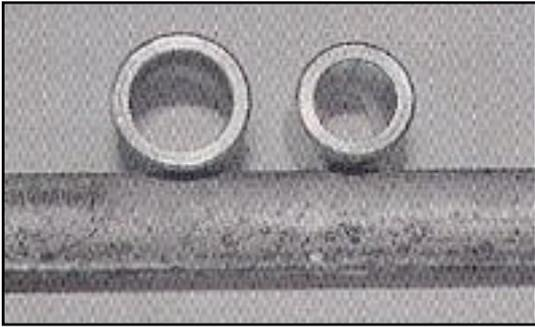
With the control arms removed, press out the old bushings. You'll notice that there's two different size spacers used for the bushings. The smaller spacers are used up front at the body mounts and the larger ones are on the knuckle. Again, lube the polyurethane bushings and install them in the arms.
