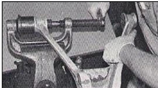
Lubricate the new polyurethane bushing and install it in the arm. Then lube the spacer and install it in the bushing.
