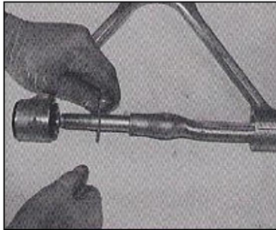
Slide the shaft through and reinstall the large and small washers into the bushing.
