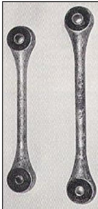
Lube the spacers and install them in the bushing. Reinstall the arms in reverse order of disassembly. Remember that the shorter arm goes on top.
