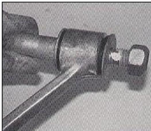
Lube and install the spacer; then install outer washer and nuts. Reinstall control arm in reverse order.
