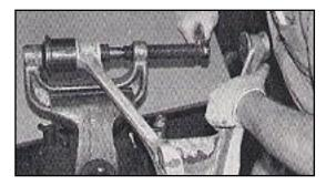
Lubricate the new polyurethane bushing and install it in the arm. Then lube the spacer and install it in the bushing.
