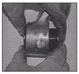
Lube the two-piece polyurethane bushing and install the side that had the larger washer (the last bushing removed). Then lubricate the spacer and isntall it in the bushing.
