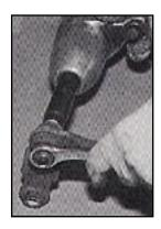
On the rear bar, you don't have to save the outer rubber bushing sleeve. Raise the rear of the car and support it, then remove the rear wheels and tires, as well as the spare tire and both upper and lower spare tire carrier. Unbolt lower sway bar end links, bolts and sway bar mounting strap bolts and remove bar from car. Remove the sway bar end links from bar.
