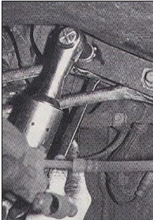
Raise the rear of the car and remove the wheels and tires. Clamp Vise Grips on the outer part of the spring and put jack stands under the spring end. Lower the car to compress the spring and remove the spring end bolt. Raise the car to take tension off the jack stand. Support the car and unbolt the upper and lower control arms.
