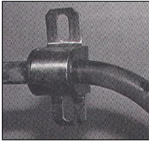
Lubricate and press in new polyurethane bushing onto the sway bar and install the spacer. Then you can lube and install the new polyurethane sway bar mount bushing and straps. Reassemble in reverse order of the disassembly process.
