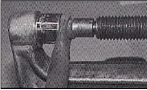
Then press out the sway bar end link rubber bushing and lube and press in the new polyurethane bushing. Also, press out the rubber sway end bushing.
