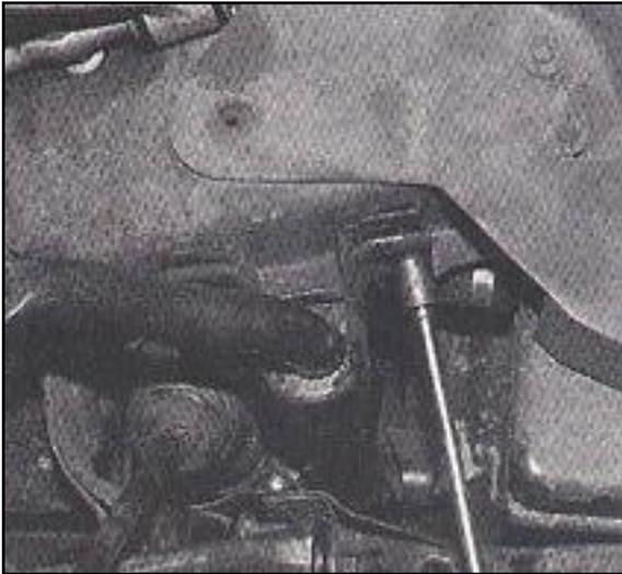
Next, remove sway bar mounting strap bolts and mounting bushing from bar and snake bar out from one side or the other. Next, remove the rubber part of the sway bar end bushing, retaining the outer steel sleeve of the original rubber bushing. You can either heat up the bushing till the rubber starts to melt, then push the bushing out or press the rubber bushing. I find using a ball joint press clamped into a vise and an appropriate sized socket works well to press the bushing.
