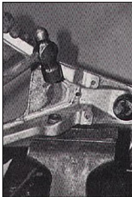
Start the bushing out with a solid rap from a hammer. Then install a socket on the bushing and knock it out the rest of the way out. Lube the polyurethane bushing and install it in the arm.
