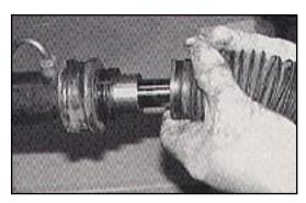
With the rack secured, cut the boot clamp and pull the boot up on the tie rod to expose the inner tie rod end.
