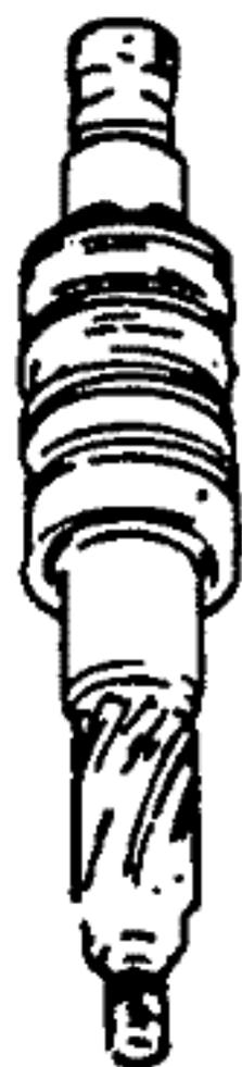
Pinion pin must not be bent, loose, or protrude beyond machined surface of valve.
