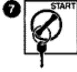
7 START Start engine. With engine idling, maintain fluid level. Reinstall cap.
