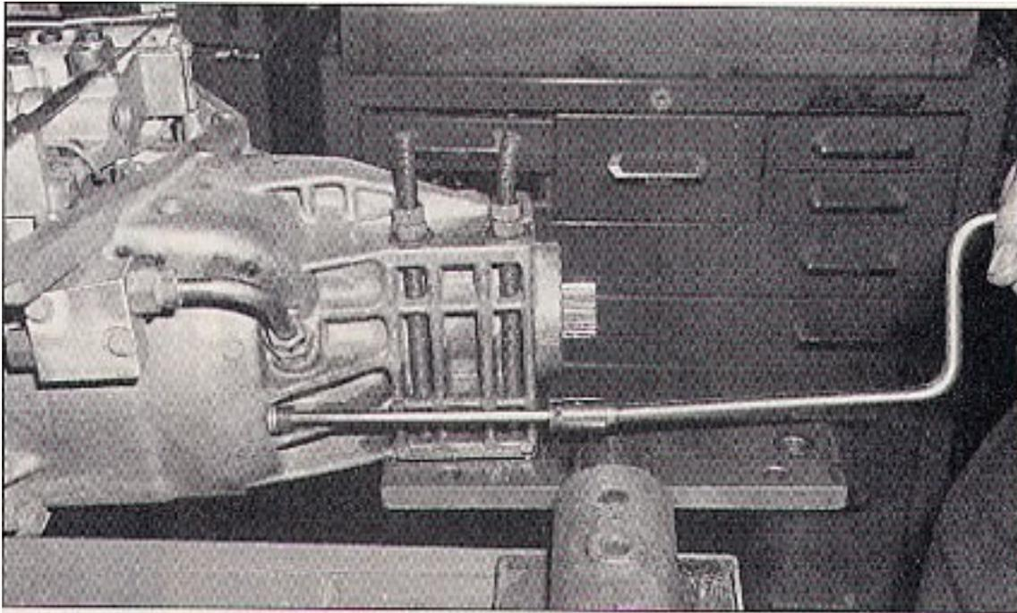
1. Remove the 3-1/8 inch pipe plugs from the rear of the overdrive unit. Install the 3 direct pressure plate retaining bolts (Part No. J-34681). Turn the bolts until they're flush with the case and then screw in two additional turns by rotating each bolt one turn at a time.
