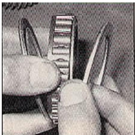
6. Assemble the output shaft and install the direct clutch sprag. If you remove the side washer on the sprag, you'll notice a shoulder on one side of the sprag. Make sure this shoulder is on the output side of the shaft when installing the sprag on the shaft.
