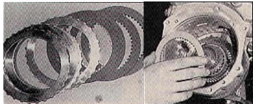
11. Alternate the remaining clutch discs and plates until all the plates and discs are installed.
