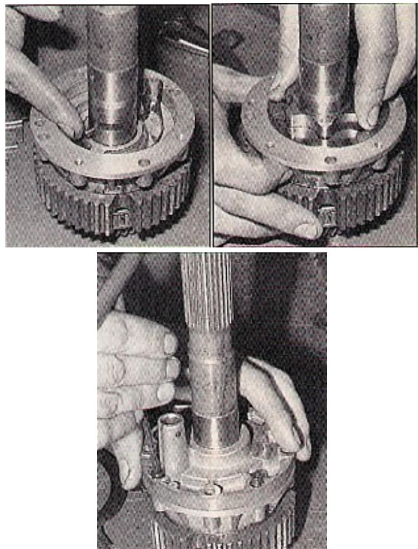
8. Install the pump housing and oil drive pin. Install the pump and pump cover. Start all four cover attaching screws, but before lightening, rotate the pump on the shaft a few times, then tighten the screws. This helps center the pump on the shaft. Now install two new O-Rings on the pump cover and the speedo drive gear.
