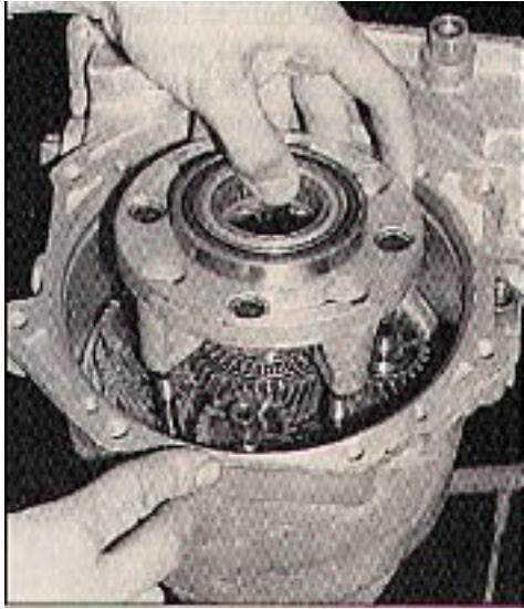
17. (right) Lower the assembly onto the direct drum bolts. The assembly should go on easily if the gears are timed correctly. Install 4 new retaining nuts and torque to specs. Check for lash in all 4 pinion gears, which indicates they are correctly timed.
