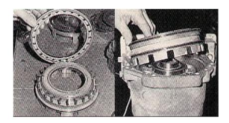
22. Install the accumulator cushion piston onto the accumulator piston and install assembly into case. Reinstall large snap ring in case making sure oil feed hold in lower right side of case is not blocked by the snap ring. Place seal protector J-34621 on input sun gear, install adapter plate sun gear seal with tool J-3423 and adapter plate O-ring, then install the adapter plate. Apply a light coating of RTV sealant on the adapter plate bolts and tighten to specifications.
