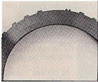
Install the direct thrust washer, installing the locking tabs into the direct apply piston. Install the thrust bearing, then the thrust washer plate which is identified from the rest of the direct plates by the tooth missing from the outer edge and a notch on a tooth on the circular ground side of the washer. This side goes down on the thrust bearing.
