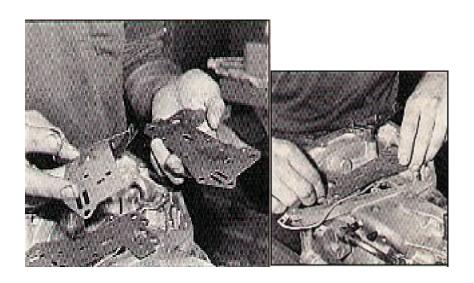
24. Install a new gasket on both sides of the separator plate and position on case.
