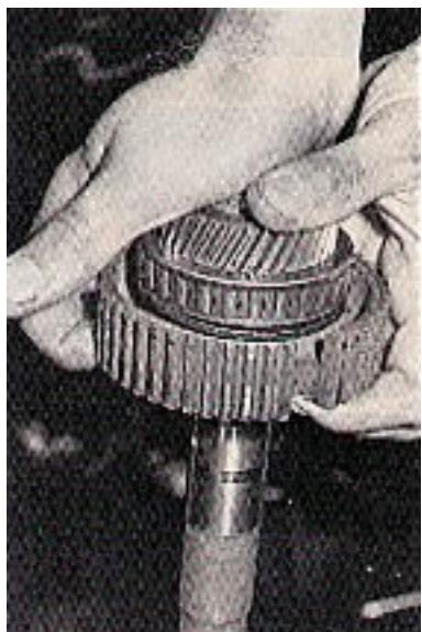
7. Install the direct clutch hub, then a hub thrust washer, then a hub thrust bearing and another hub thrust washer.
