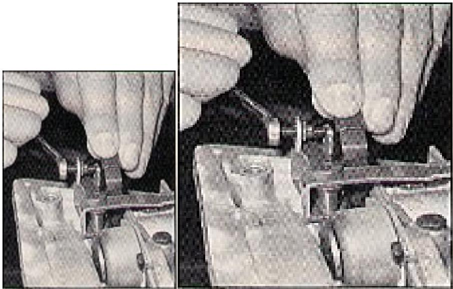
29. Next, set the hook on the lower step of the gauge. Place tool J-34671-2 between the piston and solenoid bracket. Adjust the bolt on the TV lever until the lever just touches the tool.
