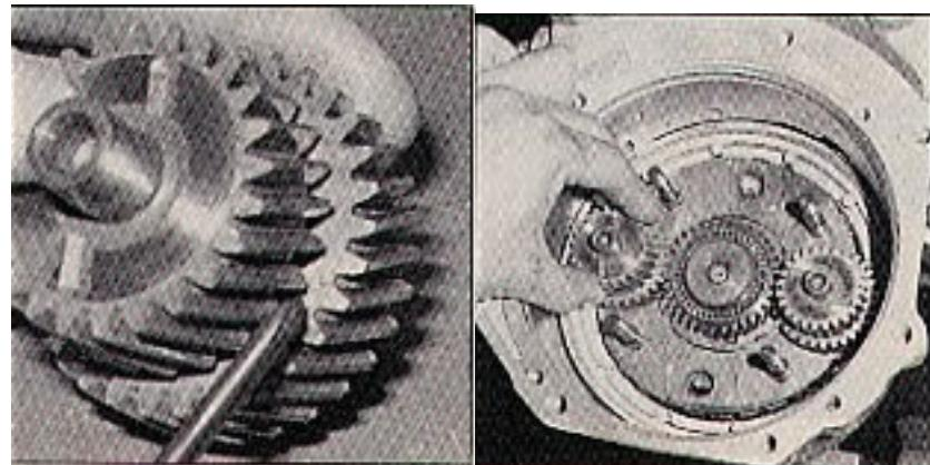
14. Install and time the pinion gears. Each gear bears a timing mark. Install the first two pinion gears opposite each other and with the mark to the center. The next two pinion gears are installed with their mark 90 degrees off center – one up, the other down. Install the output shaft thrust washer onto the bottom of the sun gear.
