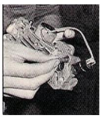
26. (right) Install check ball spring in valve body and retain with petroleum jelly.
