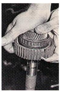
7. Install the direct clutch hub, then a hub thrust washer, then a hub thrust bearing and another hub thrust washer.
