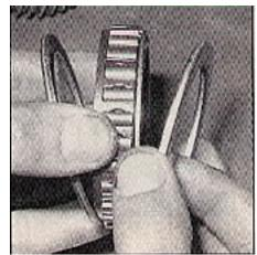
Assemble the output shaft and install the direct clutch sprag. If you remove the side washer on the sprag, you'll notice a shoulder on one side of the sprag. Make sure this shoulder is on the output side of the shaft when installing the sprag on the shaft.
