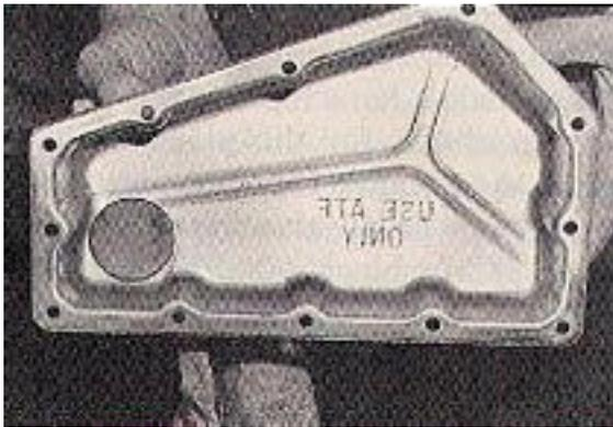
31. Install oil filter on pickup tube. Install magnet in oil pan. Apply a bead of RTV sealant to the oil pan flange and assemble wet. Install pan bolts and torque to specifications.
