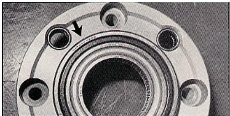
4. The annular bearing was revised in 1986 and was improved to withstand side loading on the bearing. Note the "Thrust Here" (arrow) stamped on the outer race. The early bearing was prone to failure and made a growling noise in direct drive but not overdrive. If your unit has an early direct thrust washer or annular bearing replace them with
