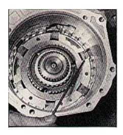
3. The old-style direct thrust washer (above right) was replaced in mid '85-early '86 with the revised washer on the left. Note the special locking tabs on the fingers that keep the washer secured to the direct piston. The problem with the old-style washer was that it would rotate from side to side and notch into the side of the case and prevent the piston from applying or releasing all the way, causing premature overdrive clutch failure.
