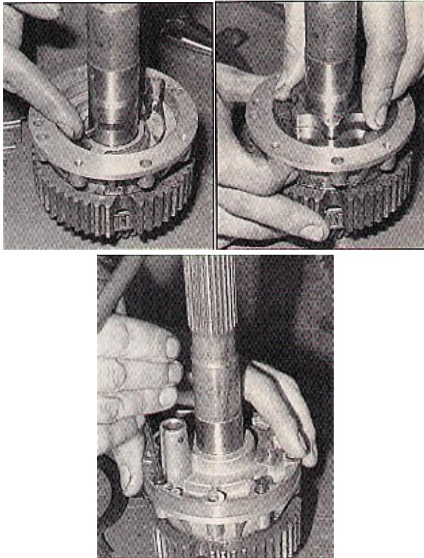
8. Install the pump housing and oil drive pin. Install the pump and pump cover. Start all four cover attaching screws, but before lightening, rotate the pump on the shaft a few times, then tighten the screws. This helps center the pump on the shaft. Now install two new O-Rings on the pump cover and the speedo drive gear.
