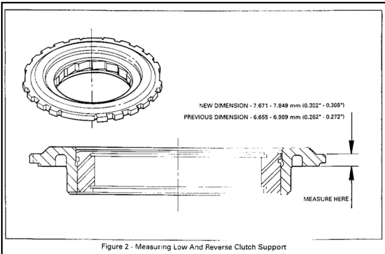
Figure 2 - Measuring Low And Reverse Clutch Support
