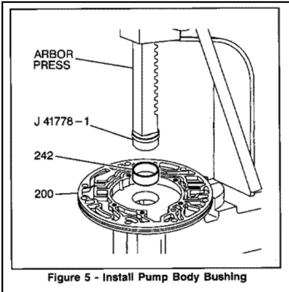
**Figure 5 - Install Pump Body Bushing**
