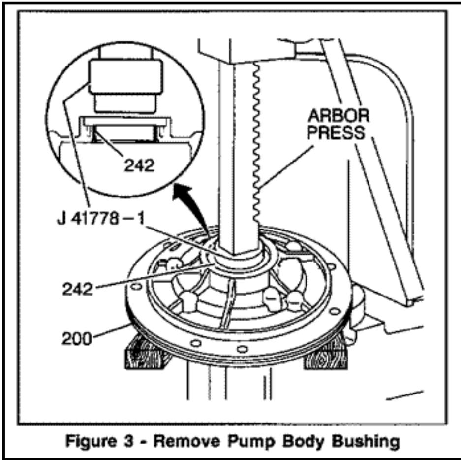
**Figure 3 - Remove Pump Body Bushing**
