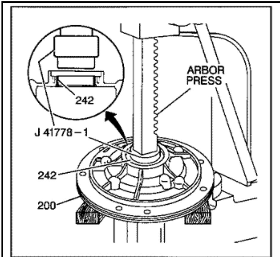
**Figure 3 - Remove Pump Body Bushing**
