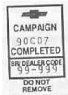
Each "Campaign Identification Label" is to be located on the radiator core support in an area which will be visible when the vehicle is brought in for periodic servicing by the owner.
