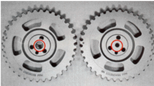
There were two cam gears used on these engines. The early ones (right) had a small hole with 16 splines for the distributor drive shaft while the later ones had a larger, unsplined hole.
