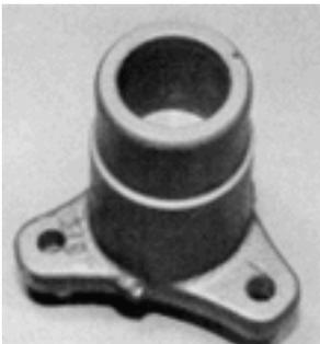
The balancer bolts onto the hub that is bolted to the crank. Note the lack of a keyway on the inside of the hub.
