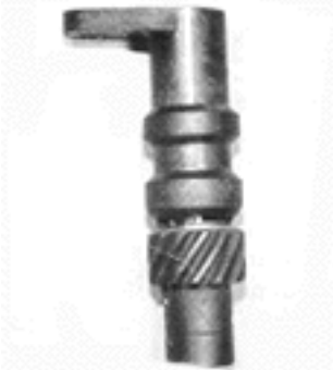
The oil pump is driven by a stub shaft that fits into the original distributor hole.
