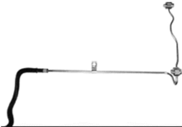
The holes in the back of the heads are connected to the reservoir with this manifold. It is needed to purge the air and steam vapors that would otherwise be trapped in the head.
