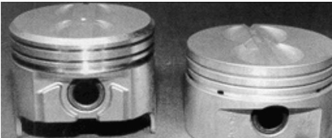
The piston for the 350 LT1 is a special, lightweight flat top with four valve reliefs. The piston for the 265 (left) looks like a smaller version of a 305.
