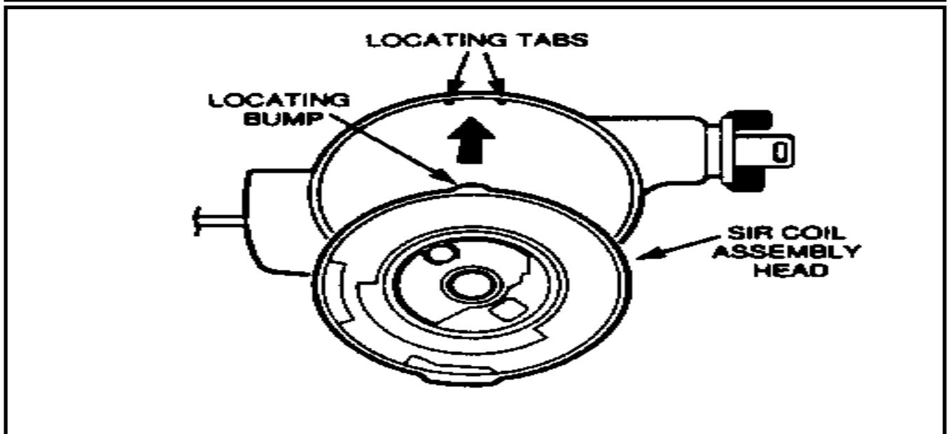
Figure 4 SIR Coil Assembly Head Seating Orientation
