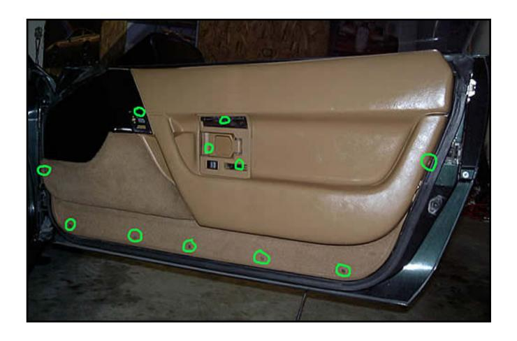
The one behind the power window switch can be reached by popping the power switch out carefully:
