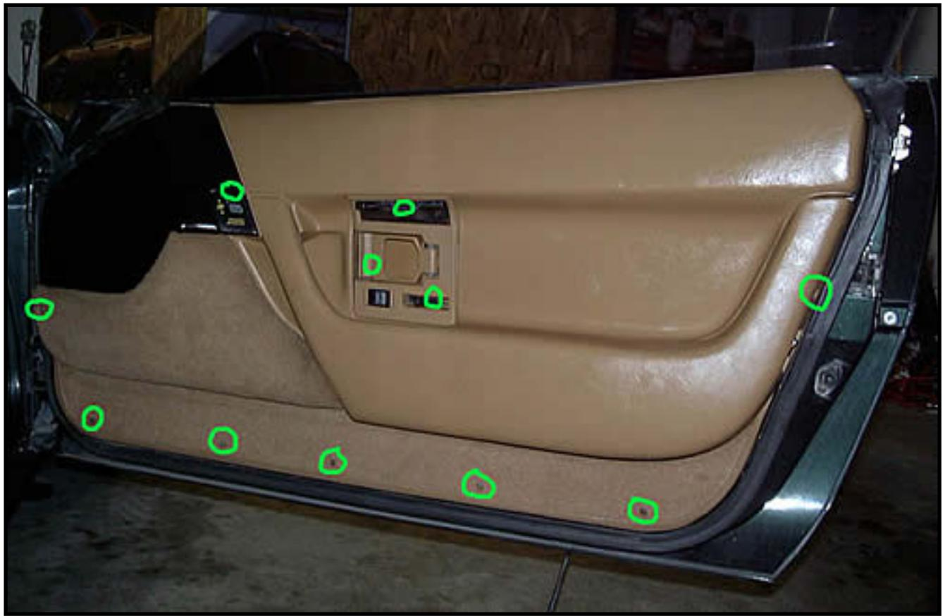
The one behind the power window switch can be reached by popping the power switch out carefully:
