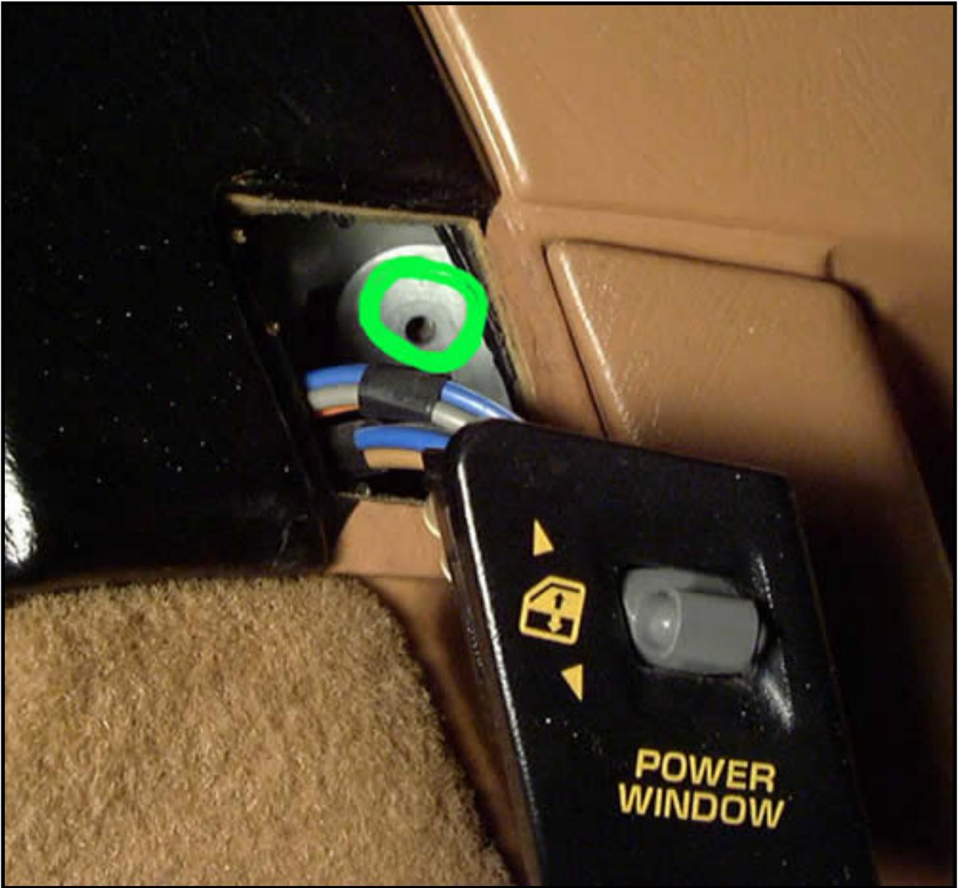
This is a closer shot of the three behind the door handle area. You'll need to pop out the light to get to the top one, and remove the plastic door lock slider piece to get the bottom one:
