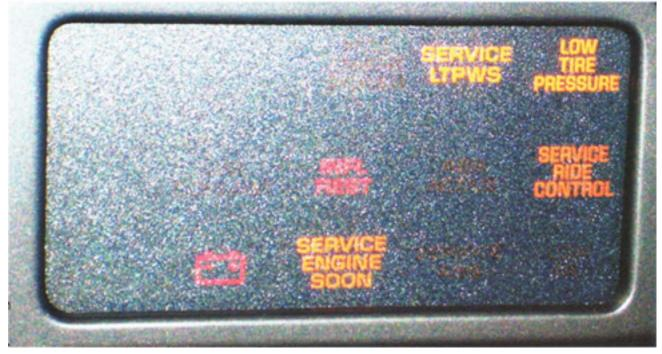
For the 1991 Corvettes, ECM and LTPWS fault codes can be read out using the same diagnostic plug from Gordon's kit, which in this case grounds Pin B to Pin A in the assembly line diagnostic link (ALDL) connector located under
