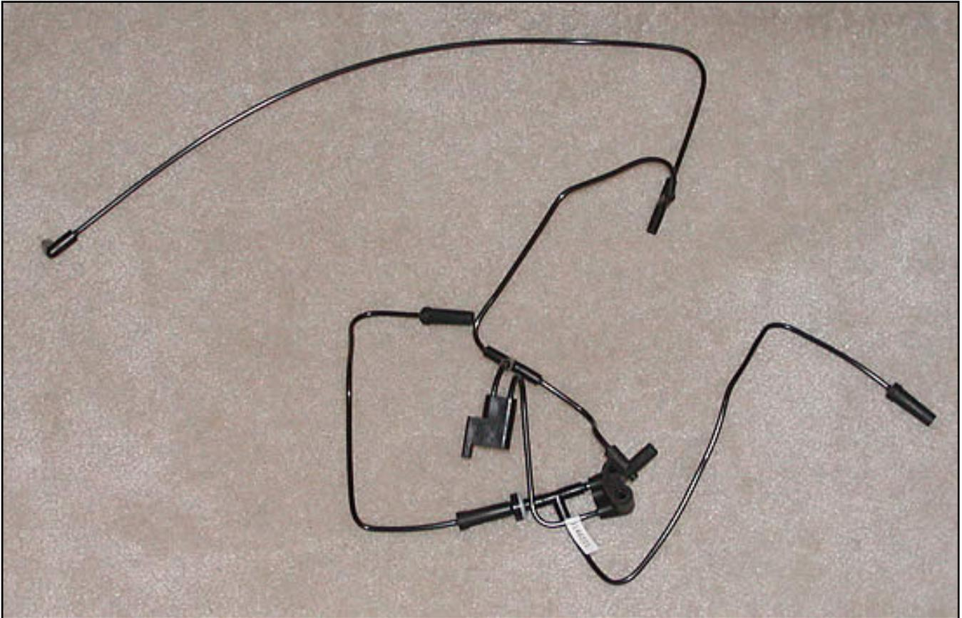
In this photo, you can see the entire secondary port vacuum hose assembly (Part #10146221). At the lower right you can see the connector that is pointed to in the picture above. The upper left hand corner connects to another connector under the ECM.
