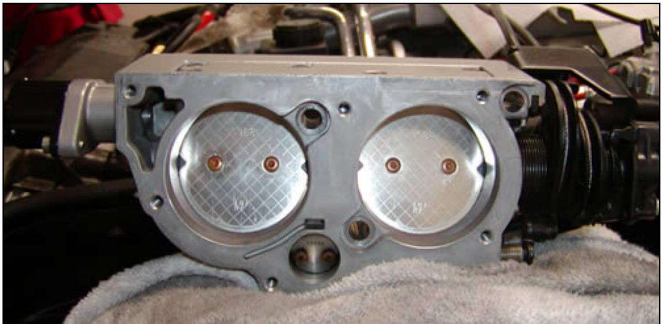
In the center of the throttle body, at the bottom, you see the primary throttle valve which is 22 mm (0.87 in.) in diameter. Above are the two larger secondary valves which are 59 mm (2.32 in.). The secondary throttle valves begin opening when the primary valve is 80% open and are completely open at full throttle.
