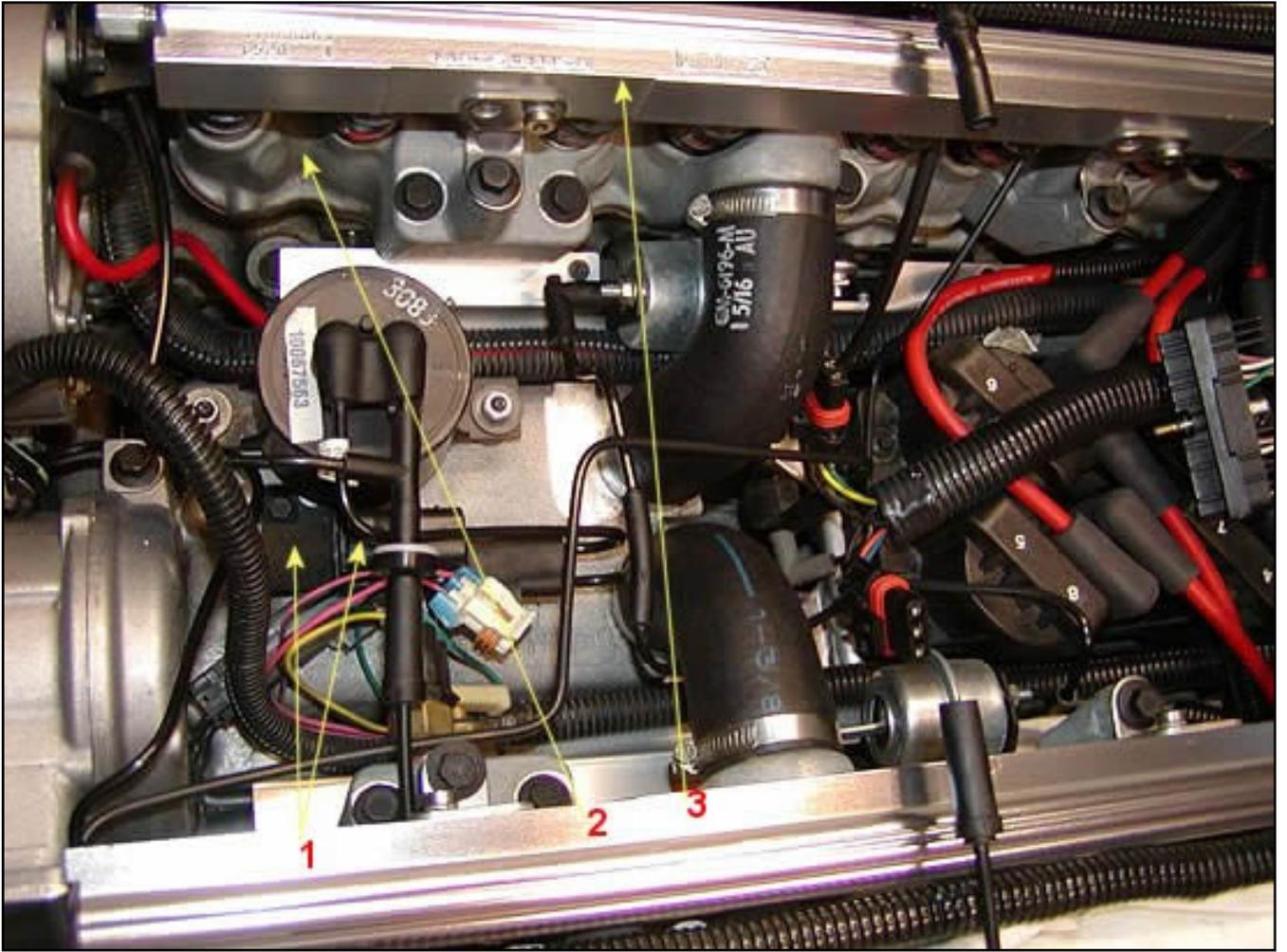
1. Vacuum Solenoid with conical air filter (Part #1997222), Conical Air Filter Part #: 10159525
