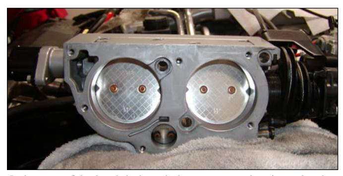
In the center of the throttle body, at the bottom, you see the primary throttle valve which is 22 mm (0.87 in.) in diameter. Above are the two larger secondary valves which are 59 mm (2.32 in.). The secondary throttle valves begin opening when the primary valve is 80% open and are completely open at full throttle.
