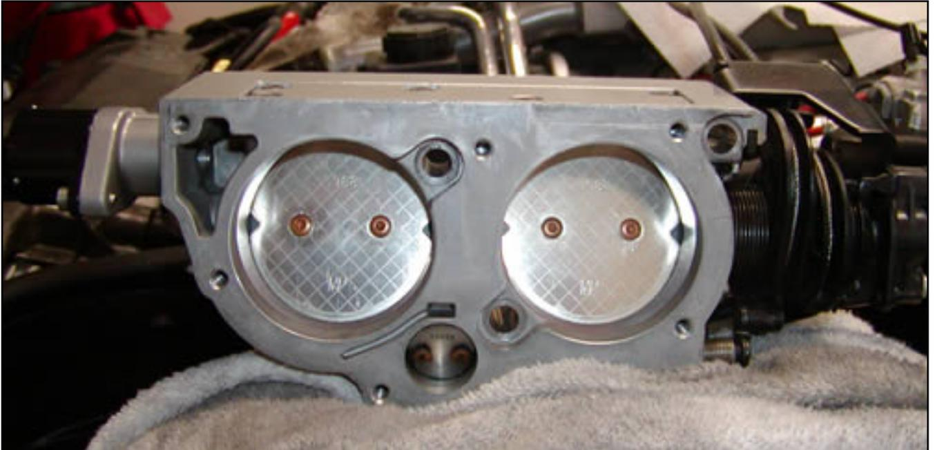
In the center of the throttle body, at the bottom, you see the primary throttle valve which is 22 mm (0.87 in.) in diameter. Above are the two larger secondary valves which are 59 mm (2.32 in.). The secondary throttle valves begin opening when the primary valve is 80% open and are completely open at full throttle.
