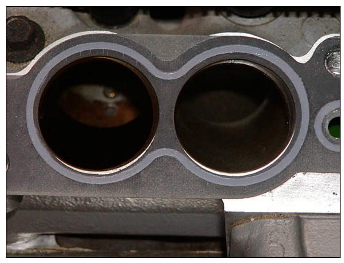
Figure 6B is a closeup view of a primary and secondary port. The primary port is on the right and the secondary port is on the left. You can see the butterfly valve inside the secondary port.
