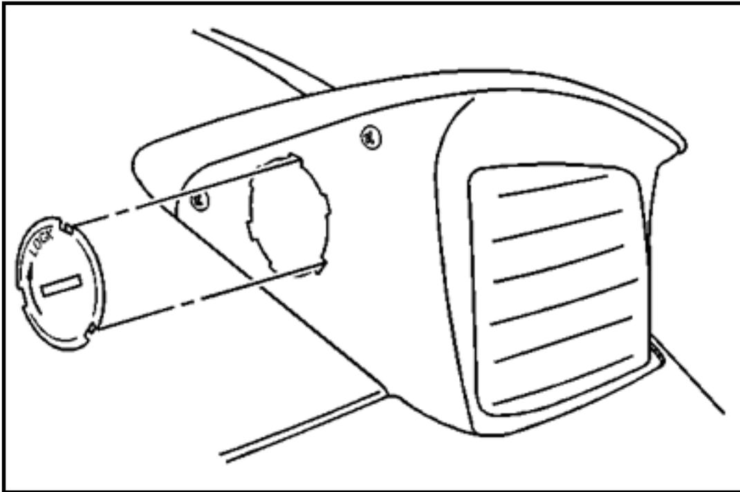
Using the following service procedure, replace both the left and right headlamp bezels with the new design bezels that have a large NOTCHED hole. The notched hole is required for installing a new design NOTCHED plug.
