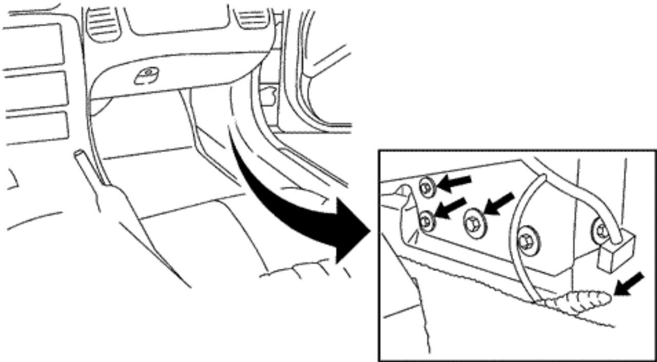
The dash attaching bolts may not be sealed. Refer to the bolts in the illustration.
