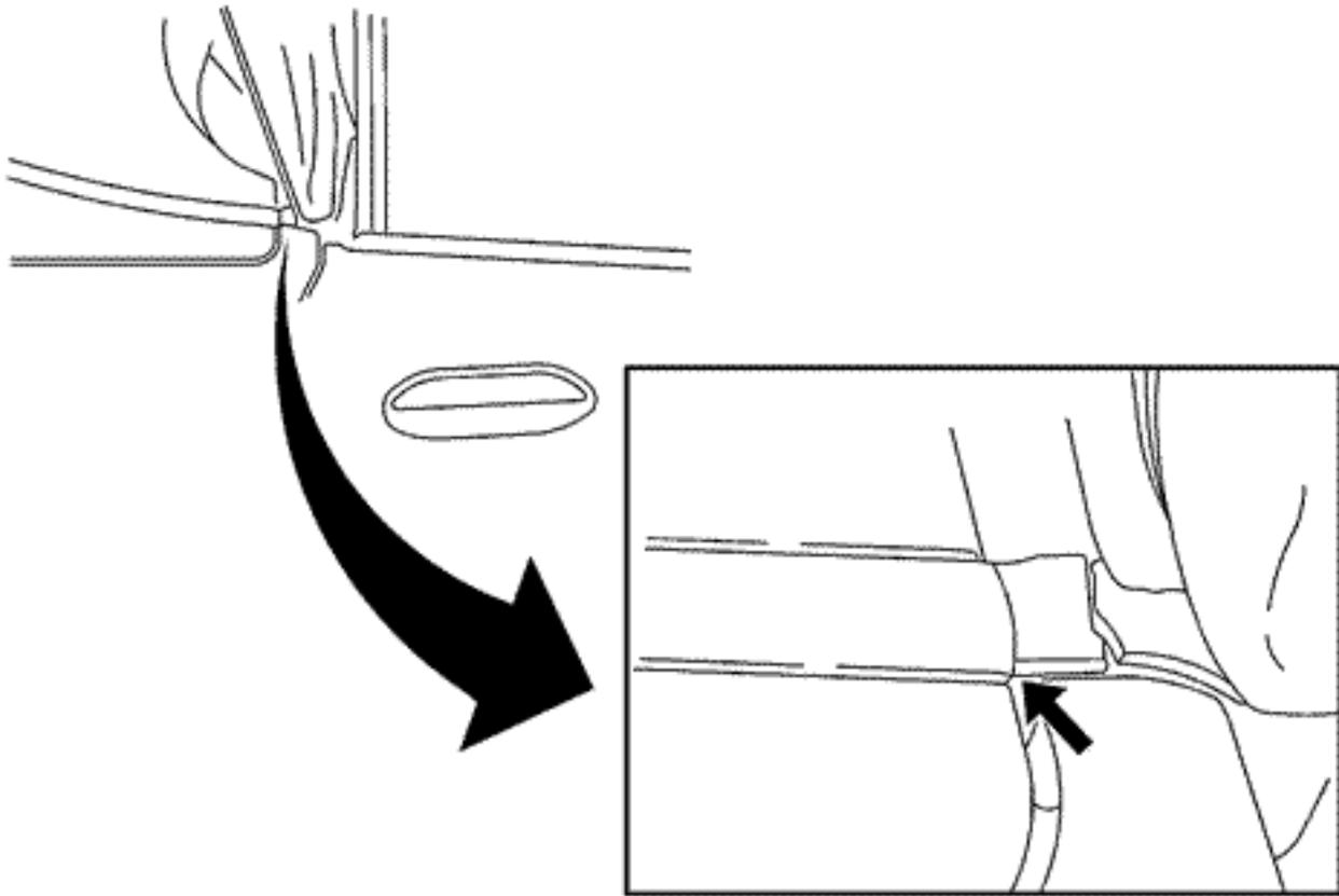
The fit where the front edge of the convertible top stowage compartment lid "protector" contacts the rear edge "bulb seal" of the "mucket"\*. Refer to the illustration above.
