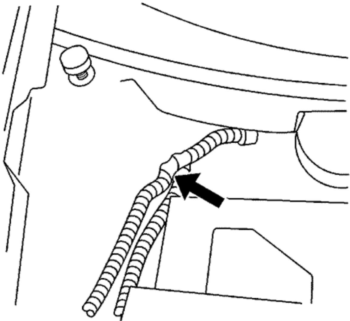
A wire harness leading into the passenger side compartment may be mis-routed (bent upward) at the first split in the wire harness. This may allow water to enter the harness and into the passenger side compartment. Refer to the arrow in the illustration.
