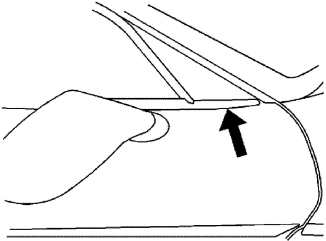
1. Verify the leak by flooding the hinge area. Refer to the arrow in the illustration.
