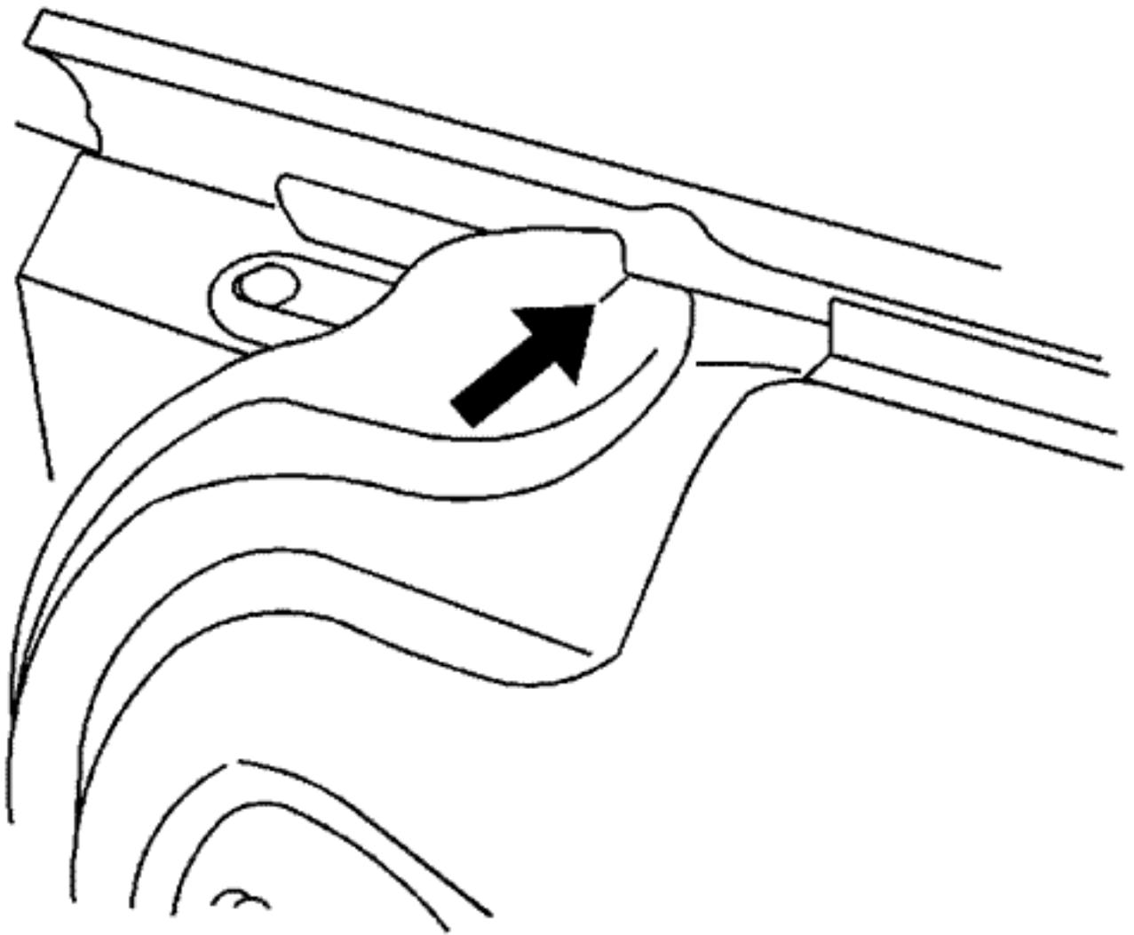
Water may be leaking around the weatherstrip at the top of the door due to an undesirable nub in the weatherstrip at the top of the door. Refer to the arrow in the illustration .
