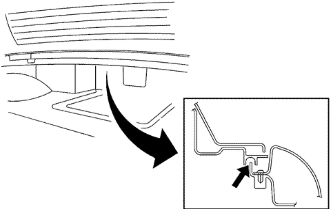
Clean the area with one of the cleaners listed below and seal the area shown in the illustration with the Kent™ sealer listed below.
