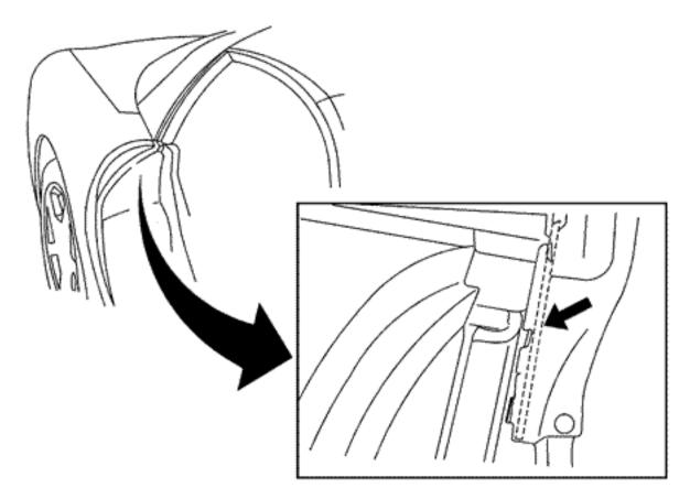
Reseal the weatherstrip with the GM sealer listed below. Refer to the dotted line in the illustration for sealing area.
