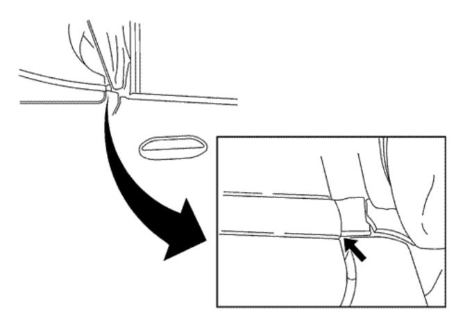
The fit where the front edge of the convertible top stowage compartment lid "protector" contacts the rear edge "bulb seal" of the "mucket"\*. Refer to the illustration above.
