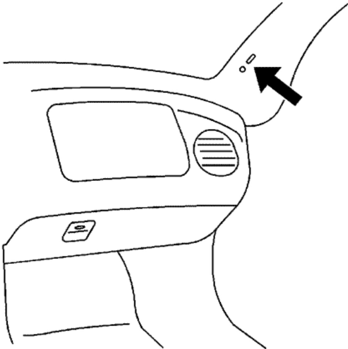
Two screws may not be sealed under the "A" pillar garnish molding. Refer to the illustration. During water test with the "A" pillar molding off, there may be water coming out of either the garnish molding retaining hole or the wire harness retaining hole. Refer to the arrow in the illustration.
