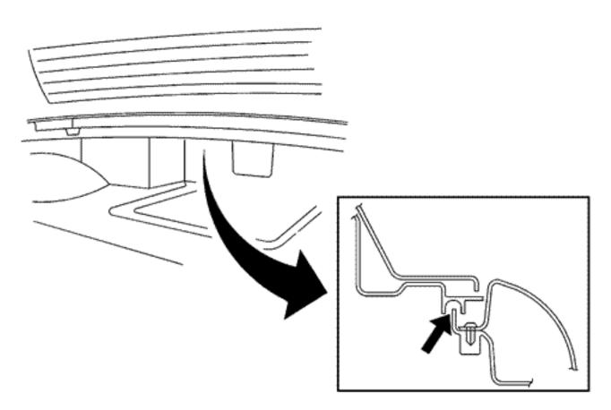
Clean the area with one of the cleaners listed below and seal the area shown in the illustration with the Kent<sup>TM</sup> sealer listed below.
