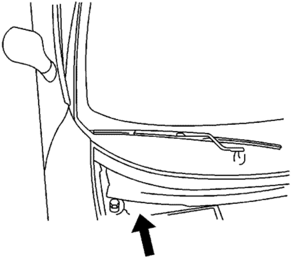
Verify the leak by flooding the front of the dash. Refer to the arrow in the illustration.
