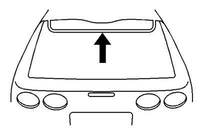
This condition may be caused by interference between the fifth bow seal and the tonneau cover rub strip. (Refer to the illustration above).
