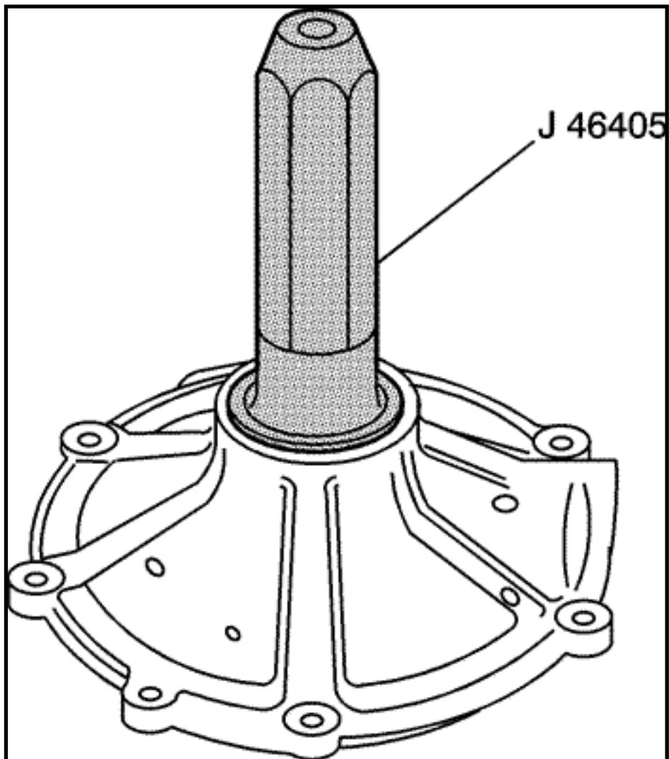
4. Install the oil seal into the cover - left using the J 46405.
