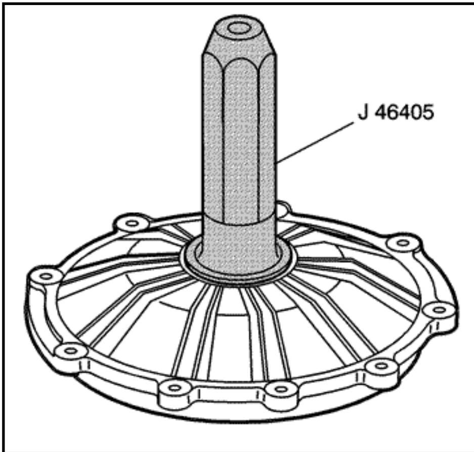
5. Install the oil seal into the cover - right using the J 46405.
