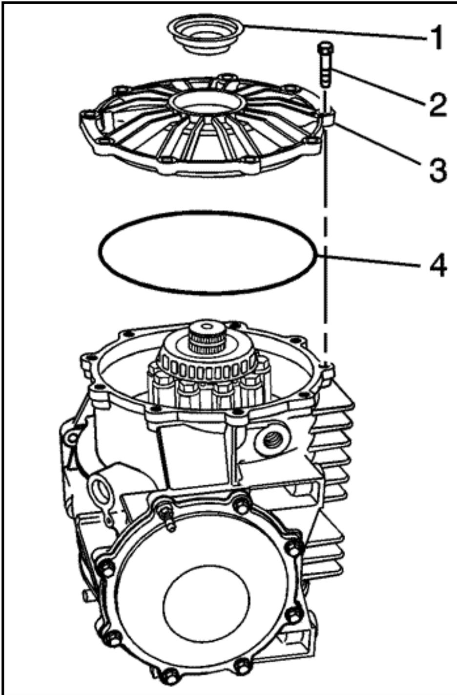
12. Install the O-ring (4) to the groove of the cover - right (3).
