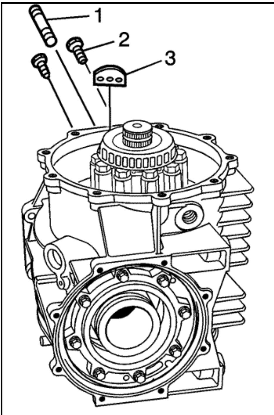
9. Apply threadlocker GM P/N 1052942 (Canadian P/N 10953466) or equivalent to the threads of the bolts (2) and stud (1). Apply threadlocker only to the end of the stud that installs into the mount.
