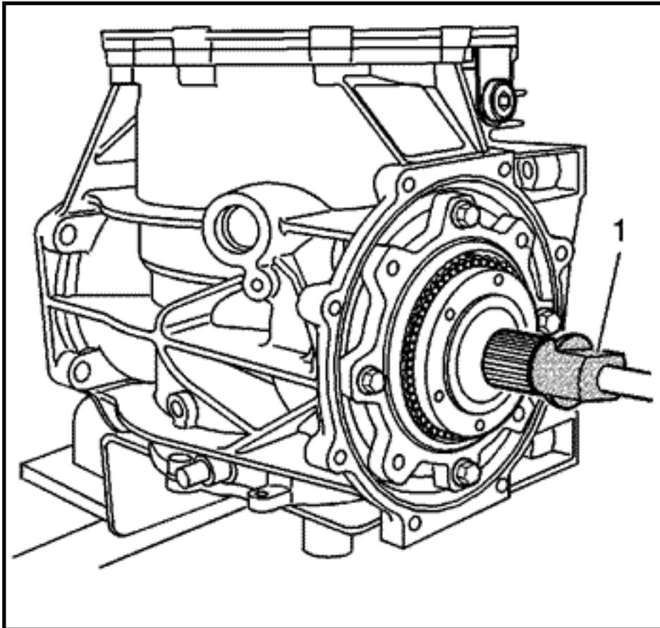
15. Install the J 42164 (1) into the splines of the pinion. J 42164 will retain the pinion in order to properly measure backlash.
