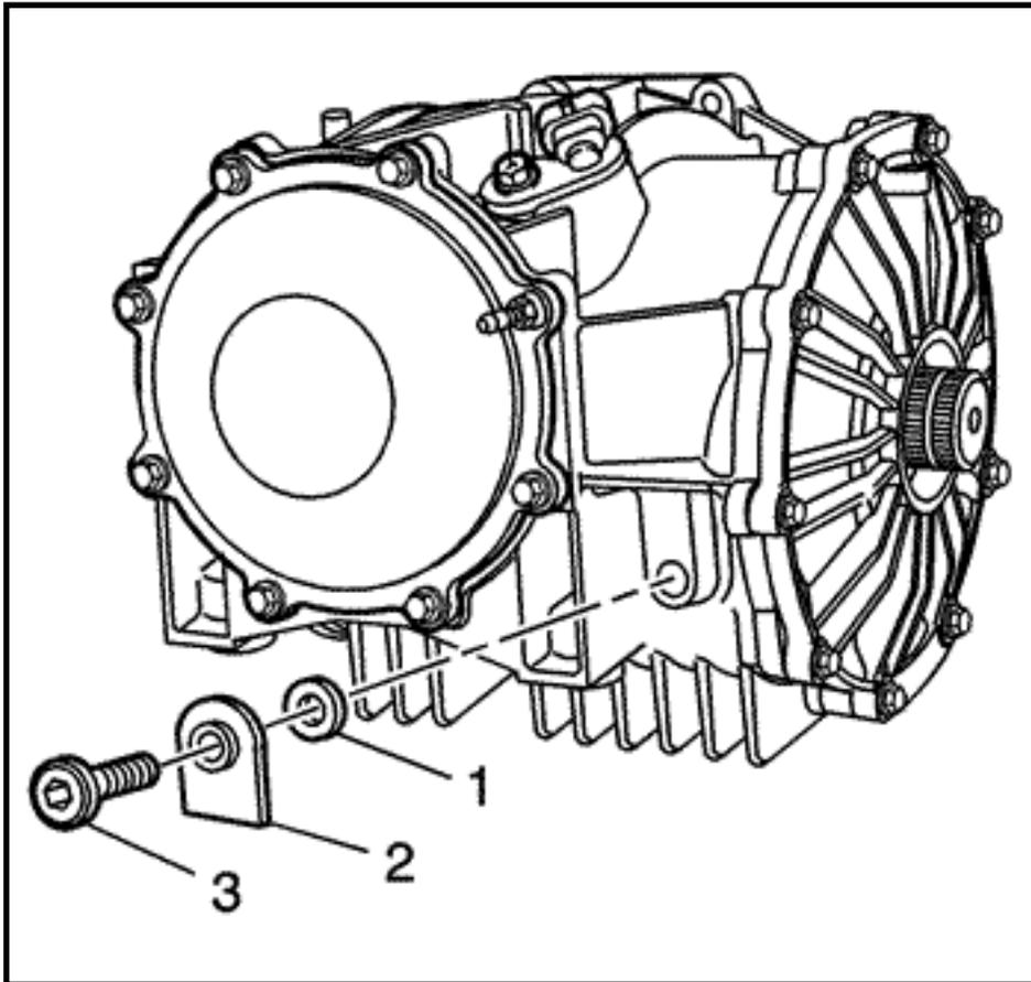
24. Install the fill plug (3), lubricant tag (2), and washer (1).
