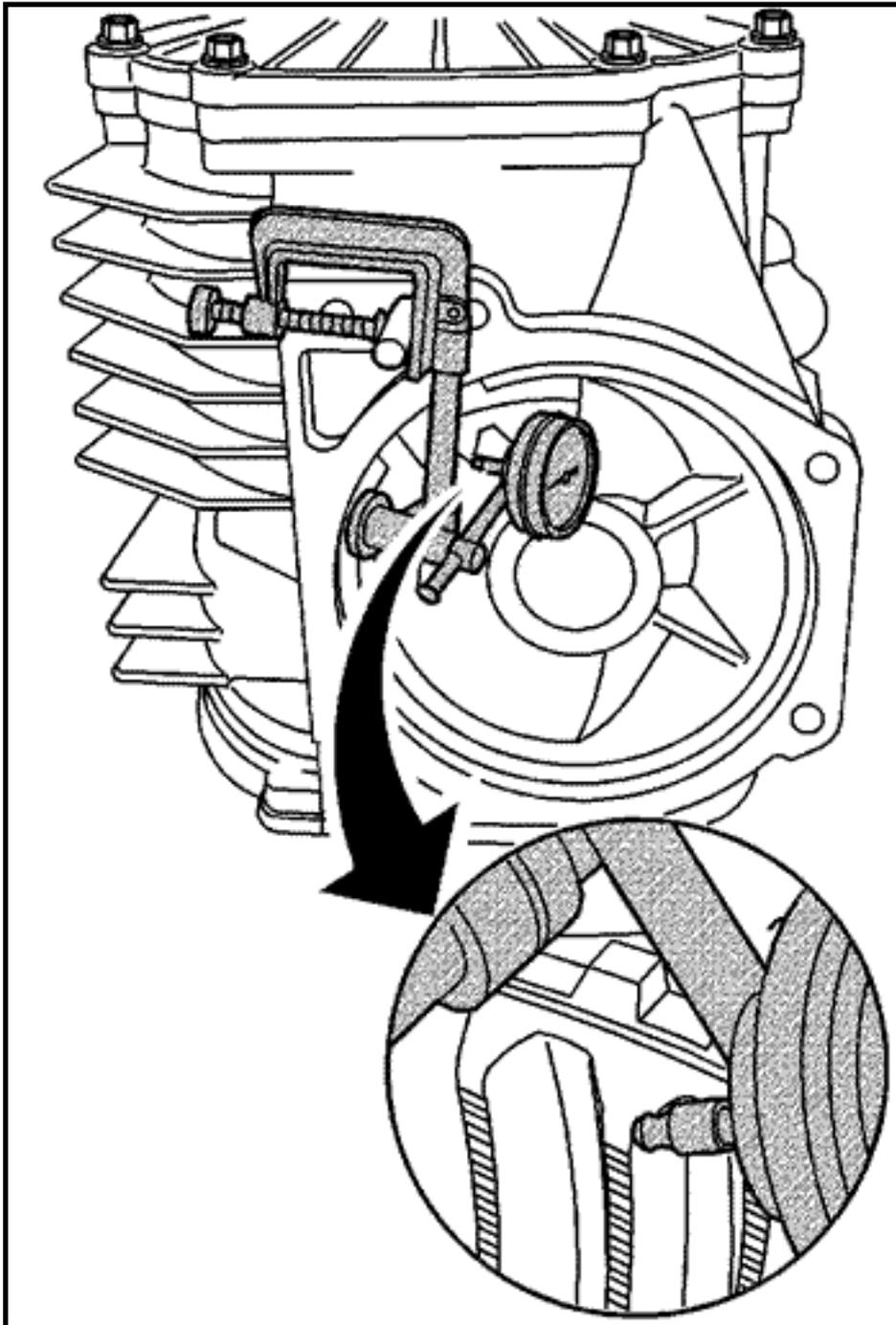
14. Install the J 8001 onto the transmission stud. Position the tip of the dial indicator against the center of the ring gear tooth surface.
