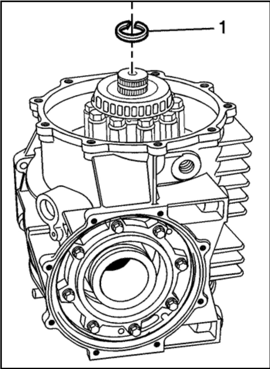
8. Install the C-clip (1) into the groove of the output shaft.
