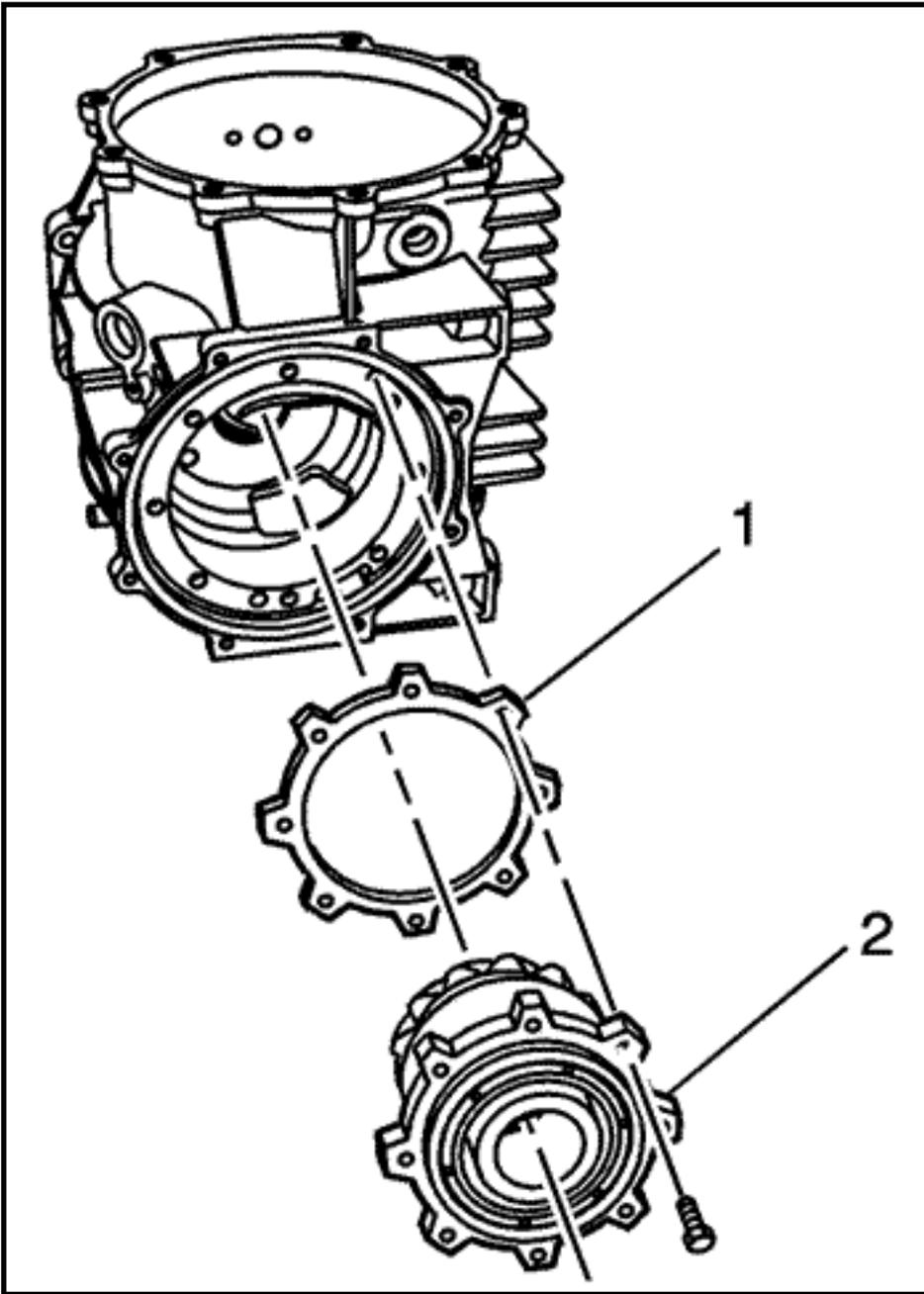
6. Install the pinion housing assembly (2) and the selected shim or shims (1) to the differential housing. Refer to Drive Pinion Shim Selection for shim selection. The use of M8 x 1.25 dowels or long bolts will ease in pinion housing/cage and shim installation and alignment.
