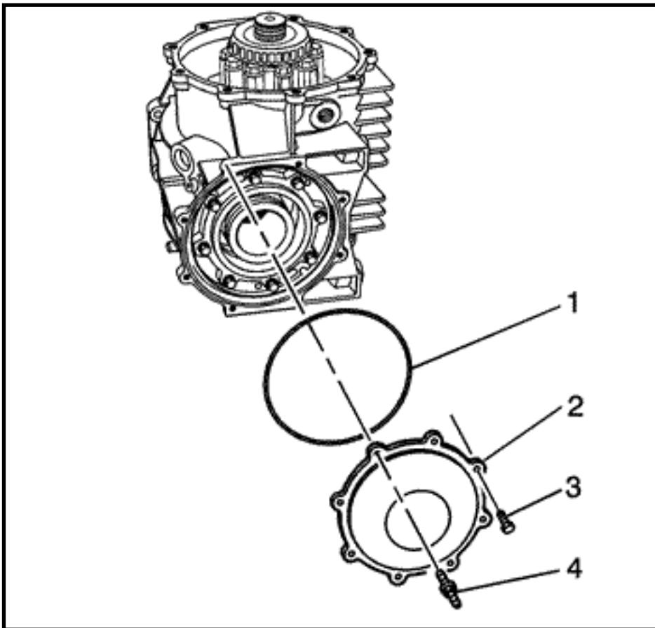
**Important** Note the location of the cover - rear bolt/stud for assembly.
