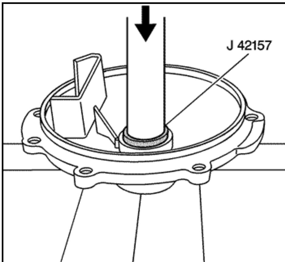
3. Install the bearing into the cover - left using the J 42157 and a hydraulic press.
