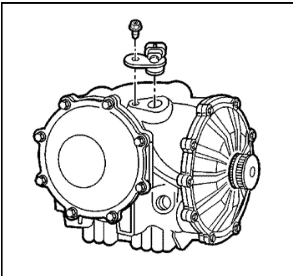
22. Install the vehicle speed sensor and bolt. **Tighten** Tighten the bolt to 25 N·m (18 lb ft).
