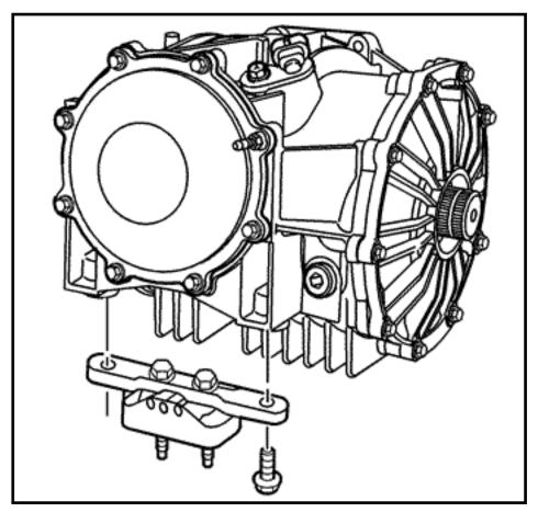
25. Install the transmission mount and bolts. **Tighten** Tighten the bolts to 50 N·m (37 lb ft).
