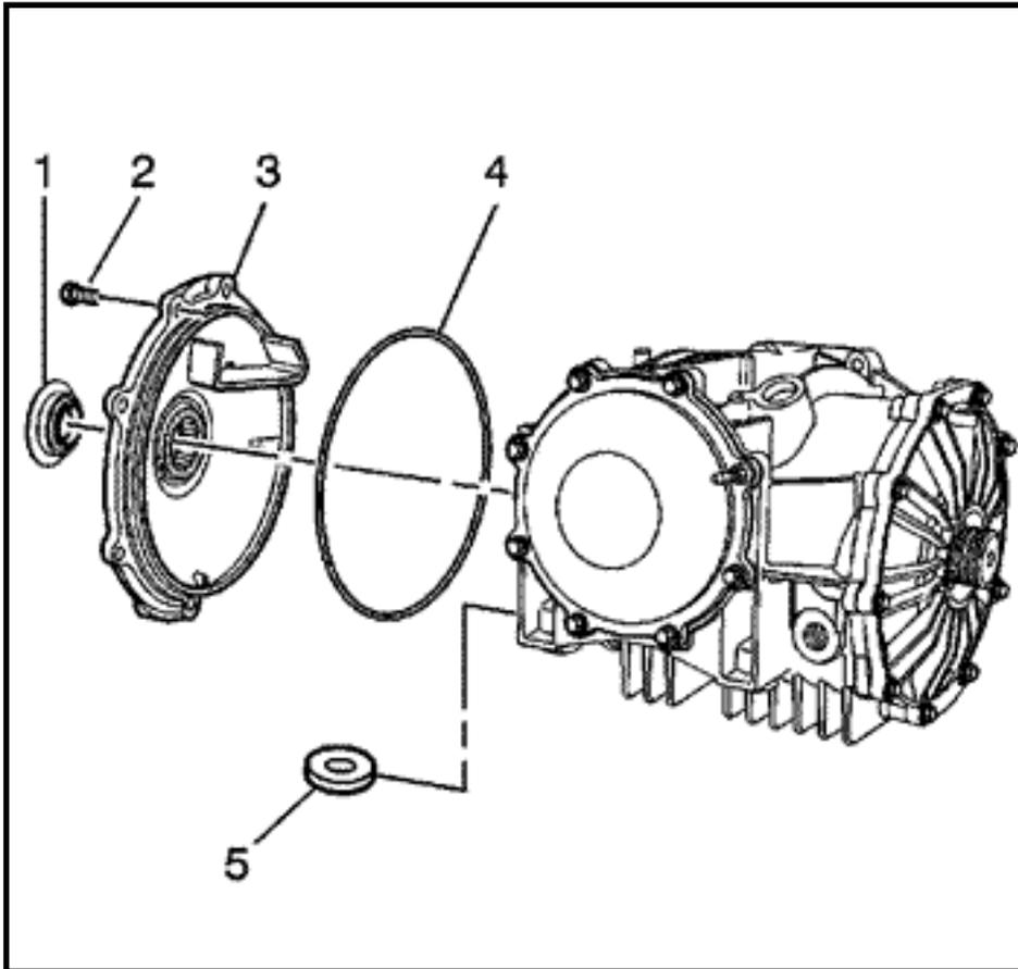
19. Install the O-ring (4) into the groove of the cover - left (3).
