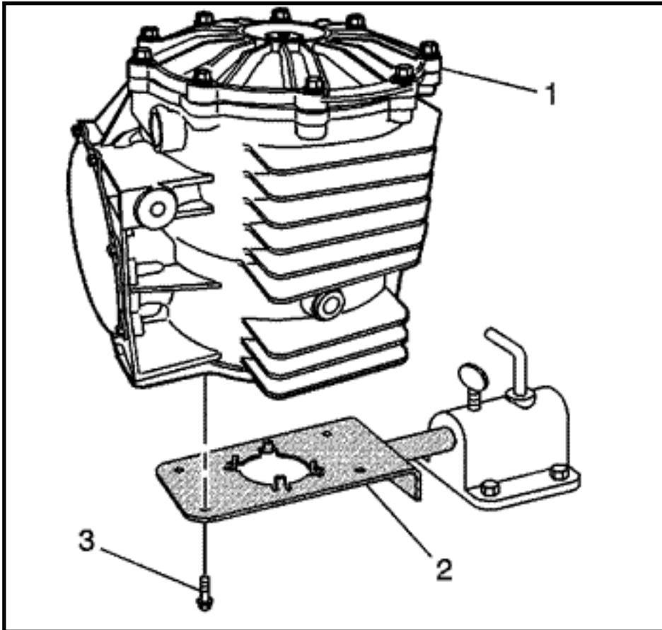
18. Remove the bolts (3) and the differential assembly (1) from the J 42173 (2).
