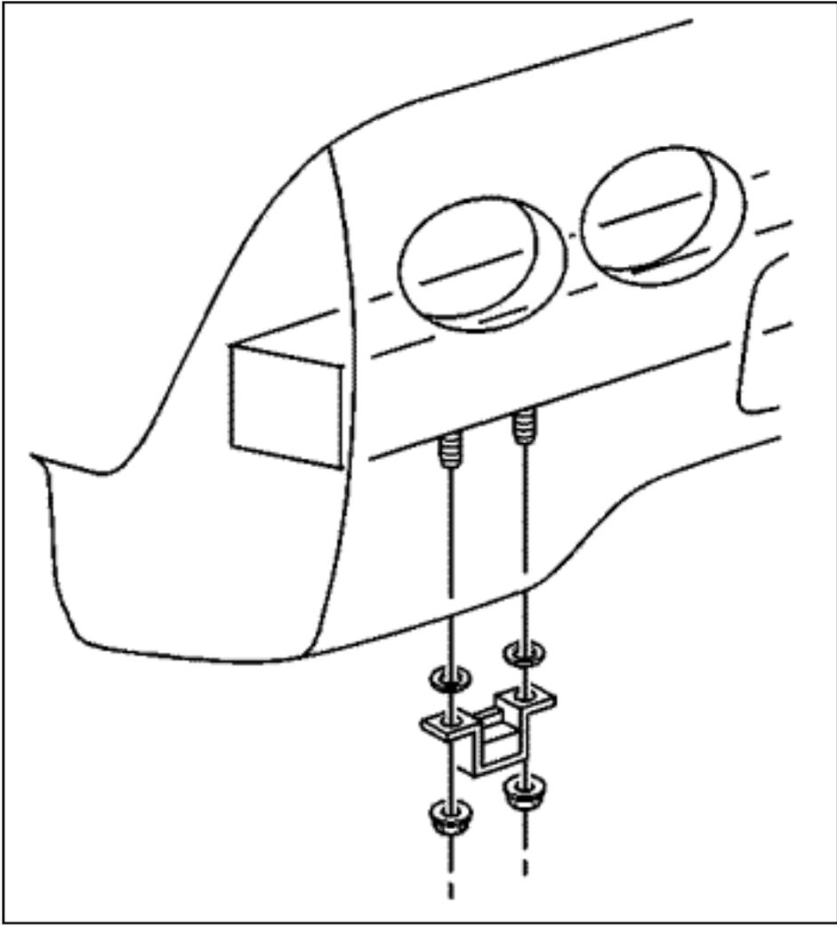
3. Insert a washer on each muffler hanger mounting stud, as shown in the figure, then raise the exhaust.
