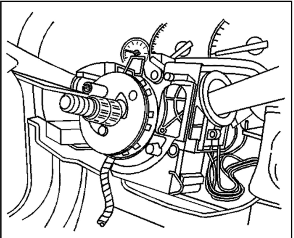
12. Remove and discard the Steering Column Lock/Cam Orientation plate
