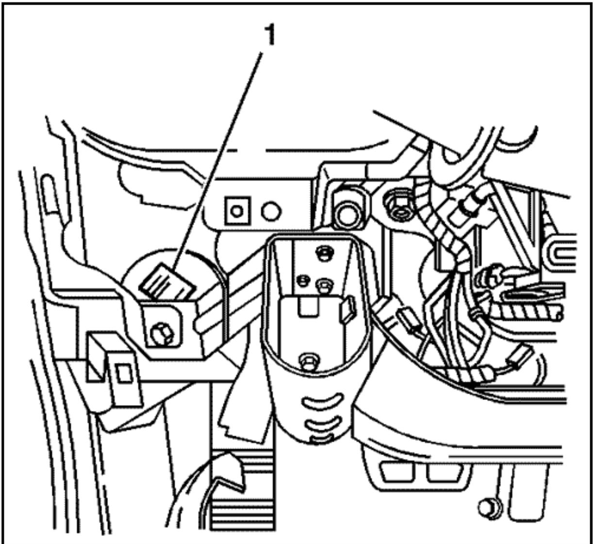
16. Route the new jumper wire and relay harness over the knee bolster (styrofoam and metal construction). The new relay (1) must be mounted to the left I/P brace with a zip tie as shown.
