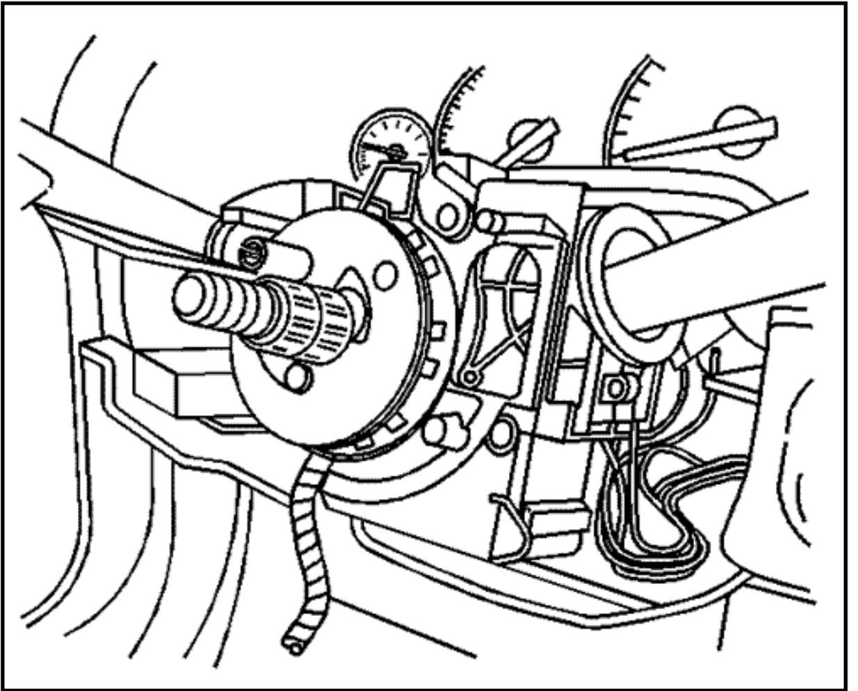
16. Disconnect the ECL electrical harness (located on the right lower side of the steering column) to the I/P main harness.
