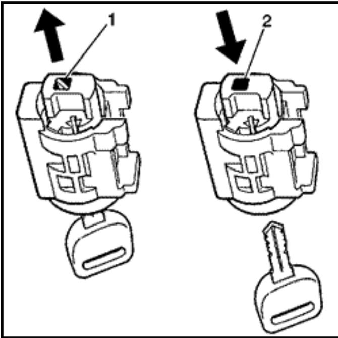
(1) Actuator in the Up Position with the Key INSTALLED in the Lock Cylinder
