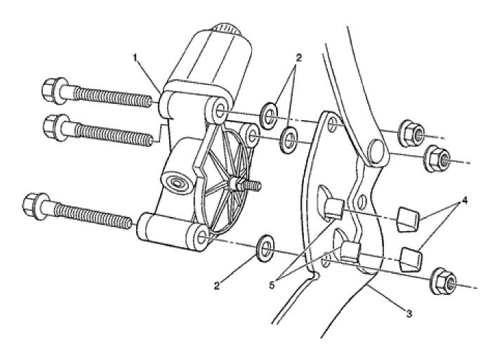
Install one washer (2) between the left headlamp door motor/actuator (1) and the mounting bracket (3) at each of the three attaching bolt locations. Also replace the insulator (4) on each of the two mounting bracket travel stop tabs (5) as shown. For information on headlamp motor/actuator removal, see the Headlamp Motor/Actuator Replacement procedure in the Lighting sub-section of Body & Accessories in the appropriate Service Manual.
