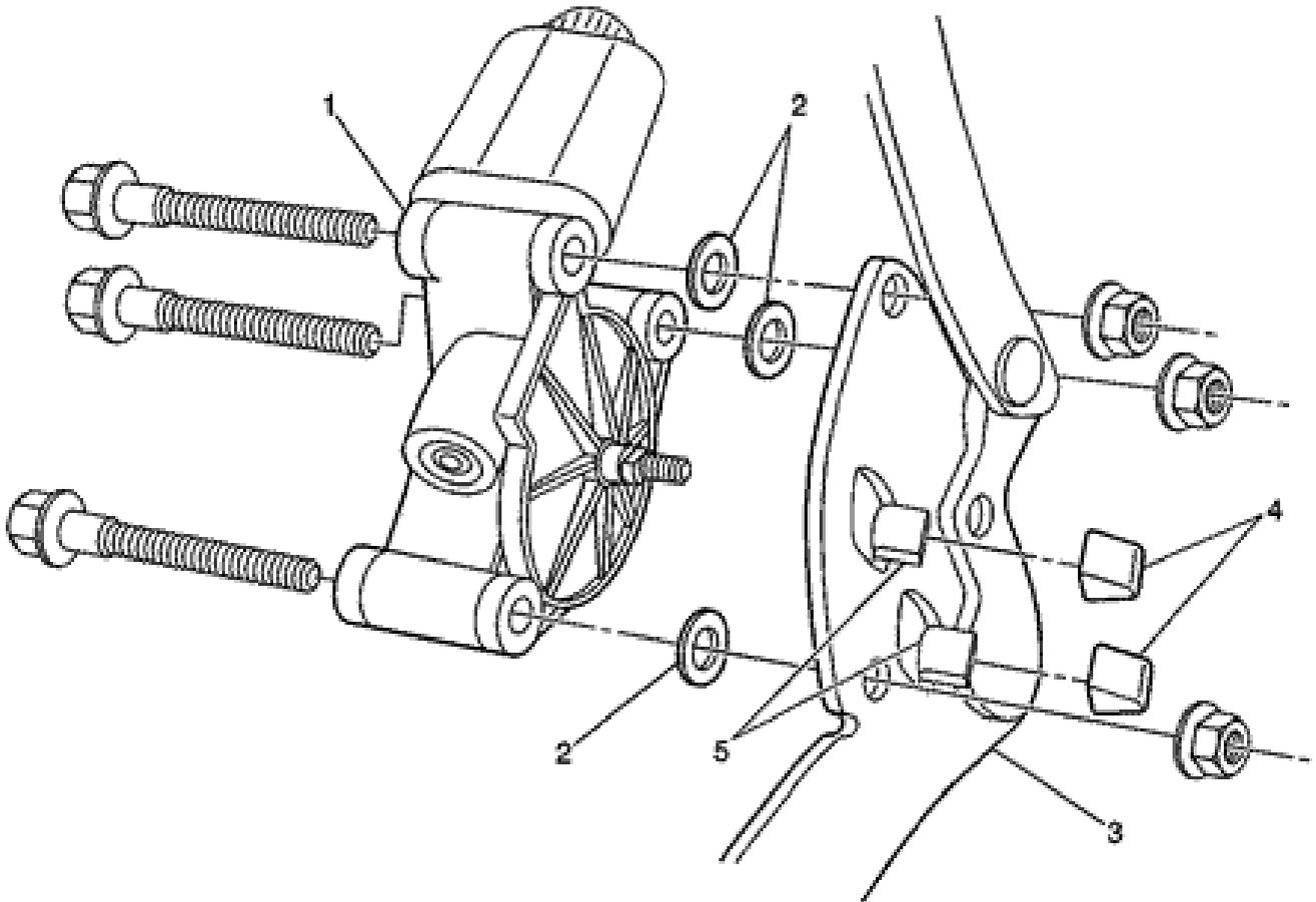
Install one washer (2) between the left headlamp door motor/actuator (1) and the mounting bracket (3) at each of the three attaching bolt locations. Also replace the insulator (4) on each of the two mounting bracket travel stop tabs (5) as shown. For information on headlamp motor/actuator removal, see the Headlamp Motor/Actuator Replacement procedure in the Lighting sub-section of Body & Accessories in the appropriate Service Manual.
