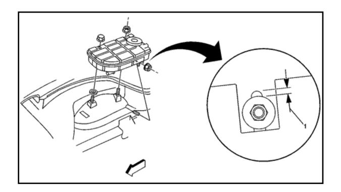
2. For all vehicles, check the level of the tank by viewing the lower mount on the tank. Less than 2 mm (.08 in) (#1) of the mounting slot should be visible above the attaching nut. If the gap is greater than 2 mm (0.08 in), loosen the surge tank and hold in a downward position to achieve less than a 2 mm (0.08 in) gap above the attaching nut. Tighten the bottom nut first, then both top nuts. **Tighten**
