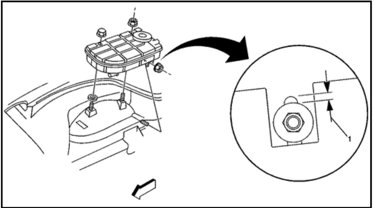
2. For all vehicles, check the level of the tank by viewing the lower mount on the tank. Less than 2 mm (.08 in) (#1) of the mounting slot should be visible above the attaching nut. If the gap is greater than 2 mm (0.08 in), loosen the surge tank and hold in a downward position to achieve less than a 2 mm (0.08 in) gap above the attaching nut. Tighten the bottom nut first, then both top nuts. **Tighten**
