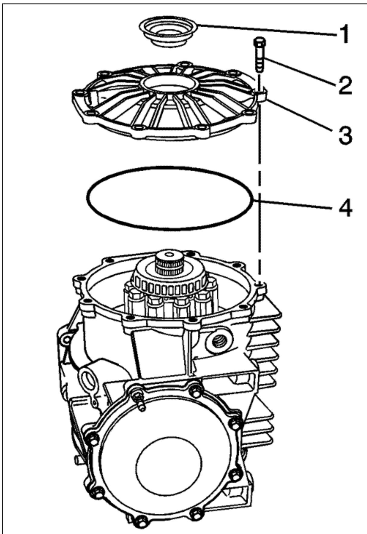
3. Clean the O-ring sealing surface on the differential cover (right) and the differential housing.
