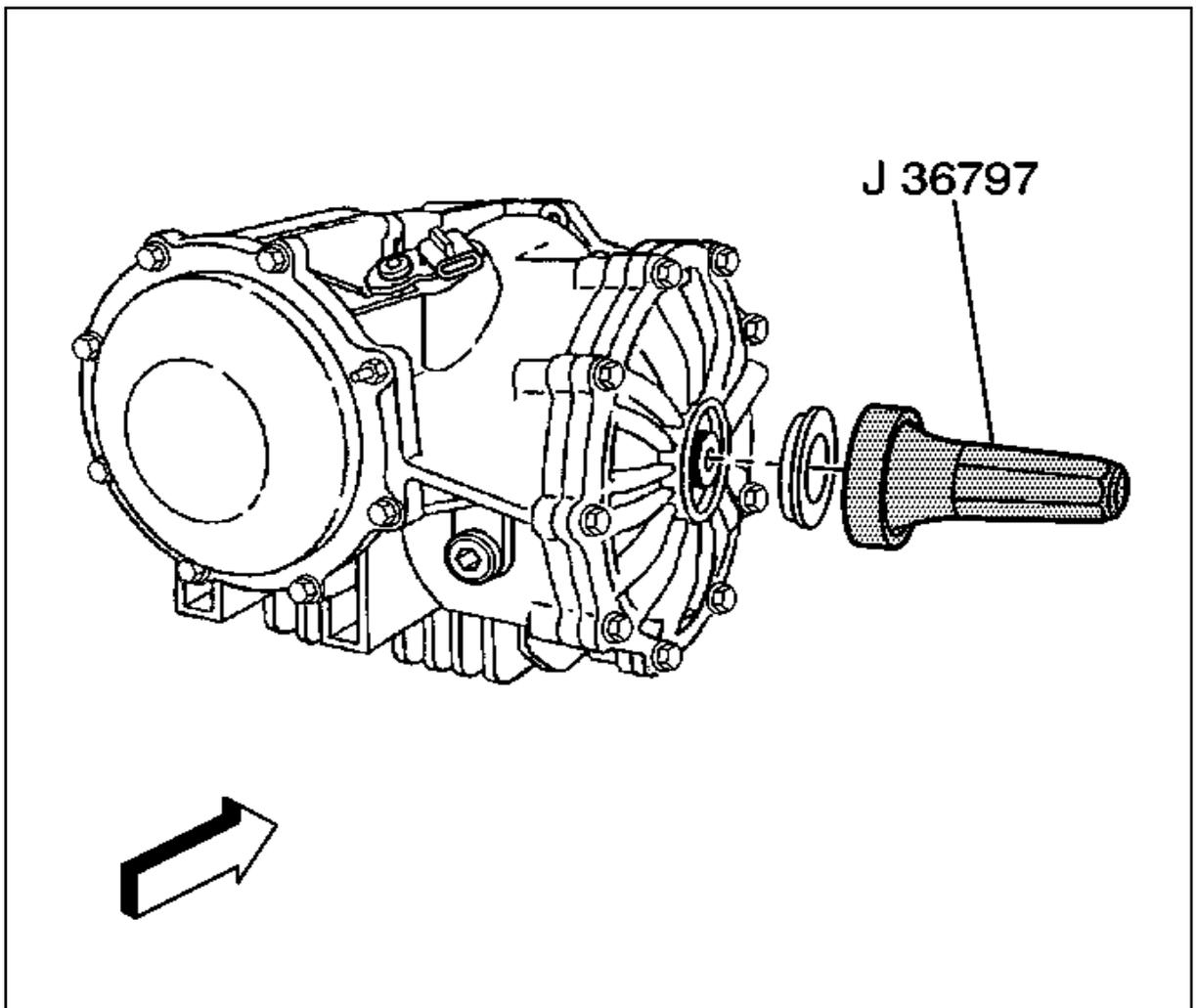
8. Install the axle seal into the differential cover (right) using J 36797.
