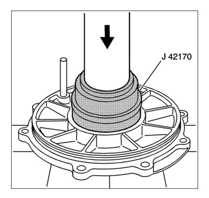
2. Press the shims and bearing race into the NEW cover (right) using the J 42170 and a hydraulic press.
