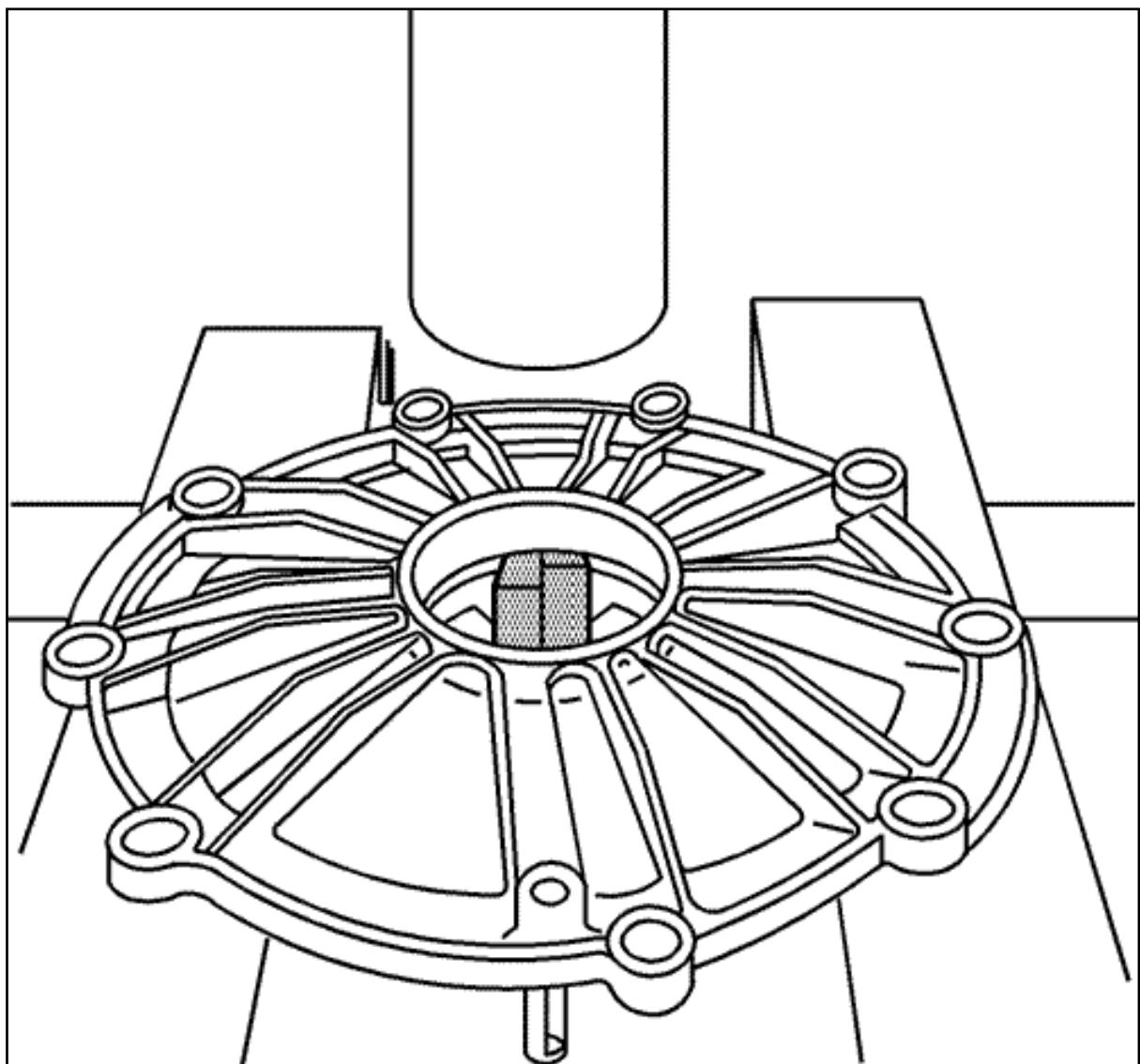
11. Install the J 42194 into the differential cover (right), in order to remove the bearing race and shims. Position the cover into a hydraulic press.
