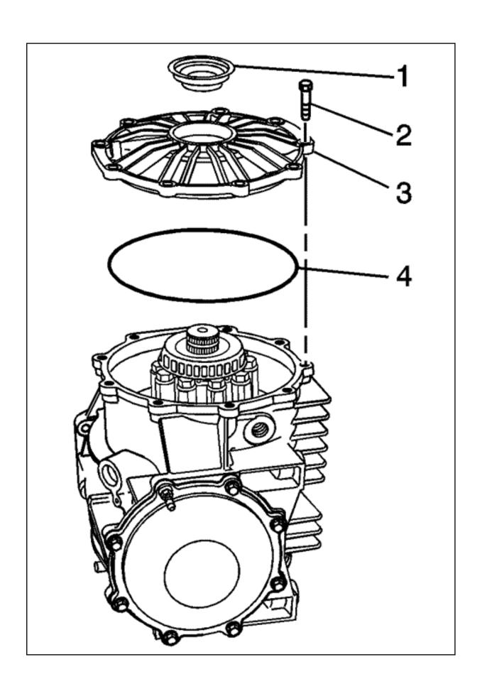
10. Remove and discard the axle seal (1), and O-ring seal (4) from the differential cover (right).
