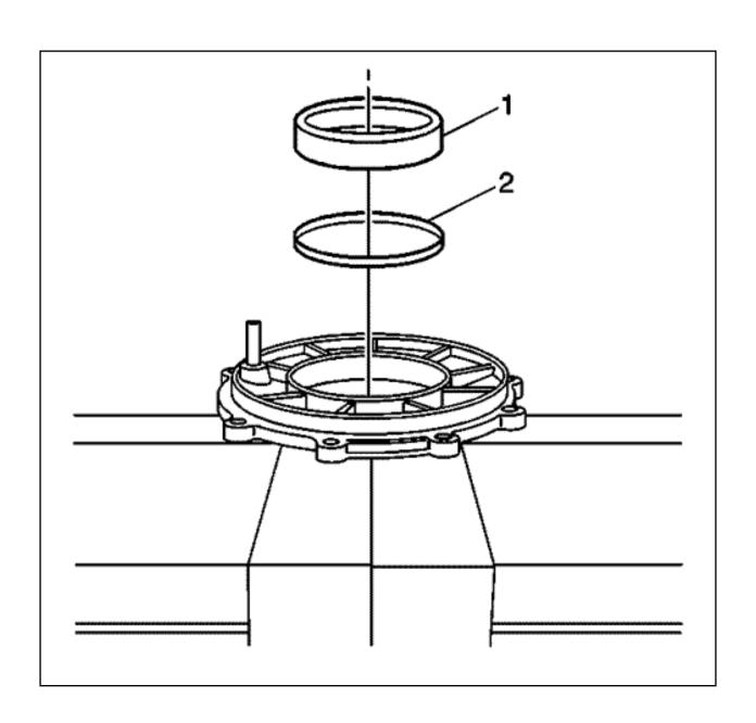
12. Using a hydraulic press, remove the bearing race (1) and shims (2). Mark or tag the shims for assembly.
