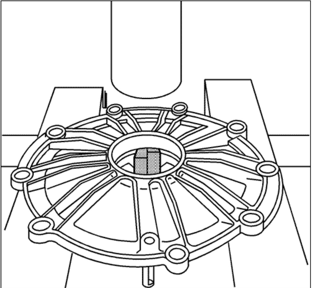
11. Install the J 42194 into the differential cover (right), in order to remove the bearing race and shims. Position the cover into a hydraulic press.
