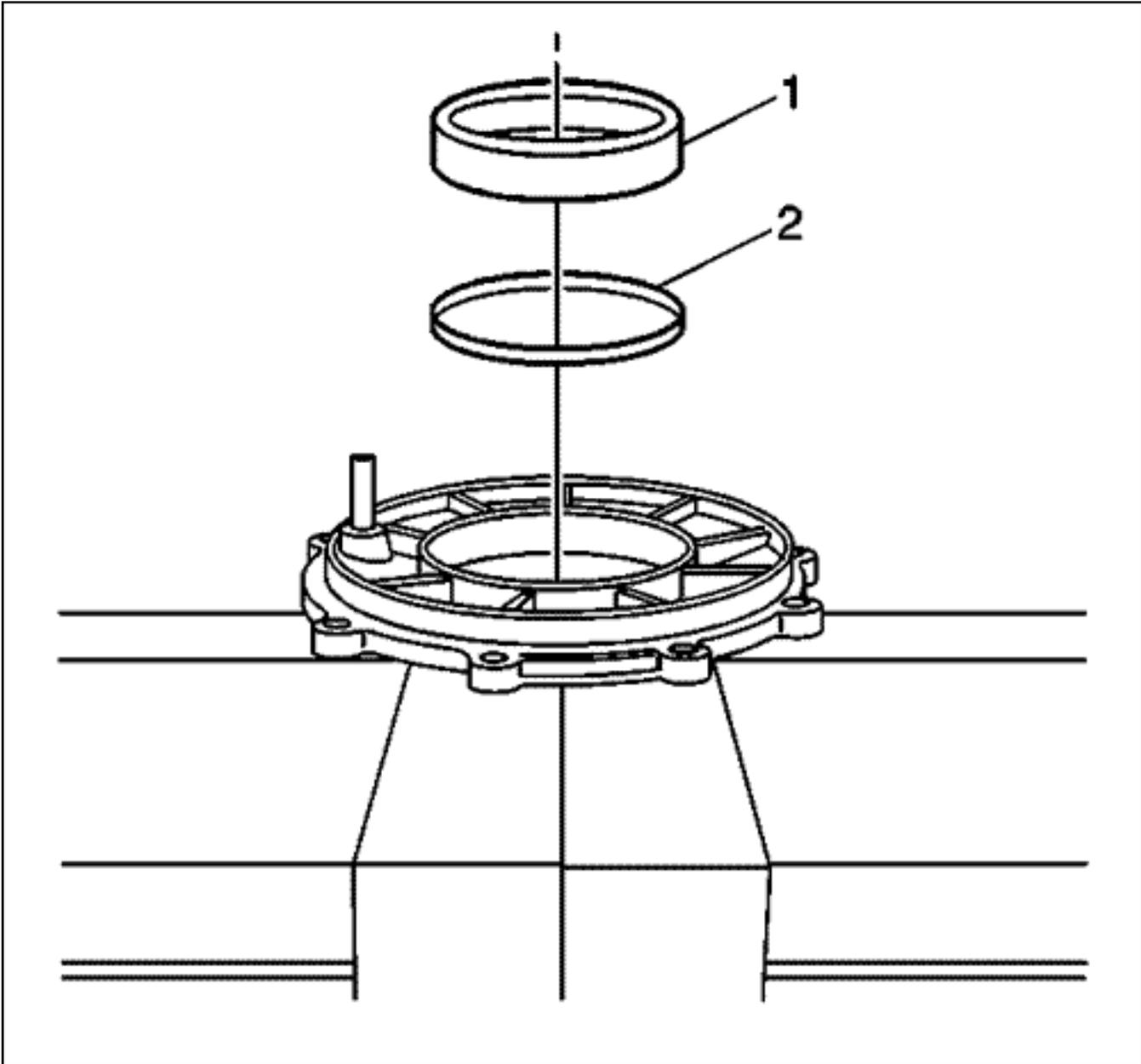
1. Install the selected shims (2) and the bearing race (1) to the NEW cover (right).
