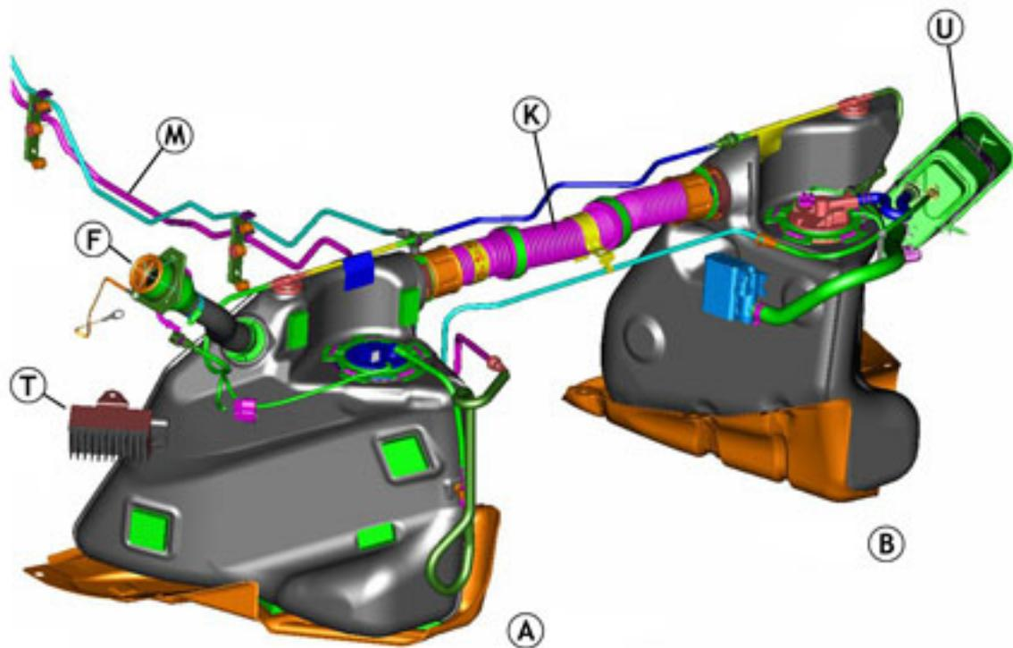
Each tank contains a sensor module, which includes a float and resistor card.
