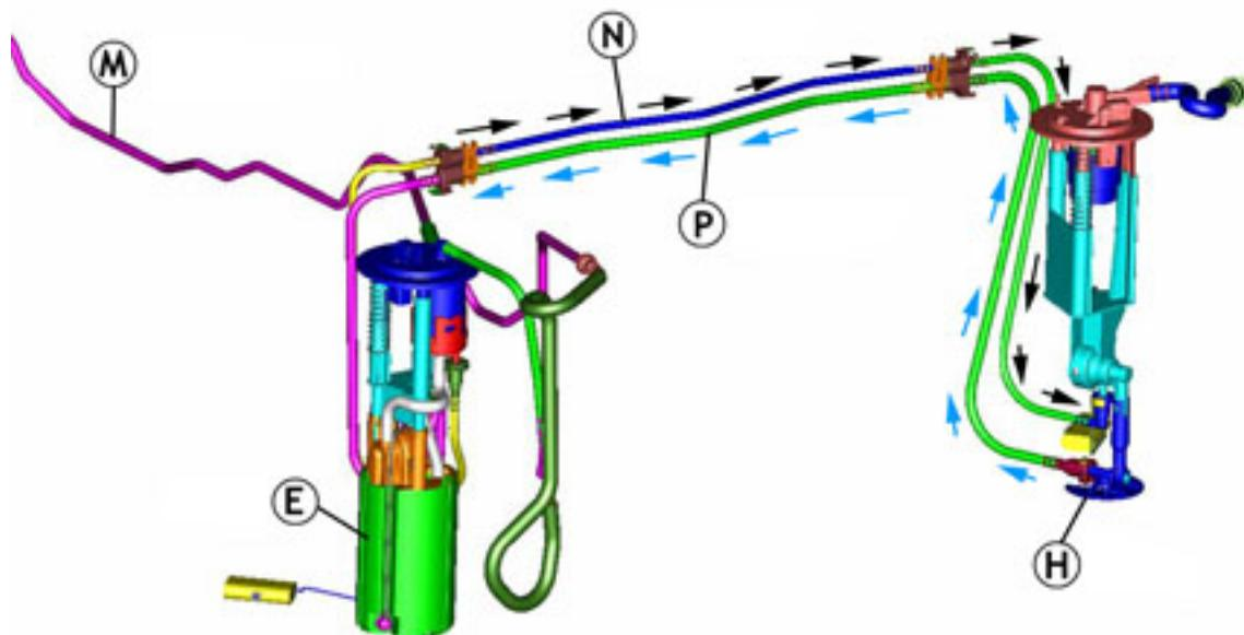
**TIP:** The pressure regulator is in the fuel tank, not on the fuel rail on the engine. This type of fuel system is called returnless, or demand. This means that
