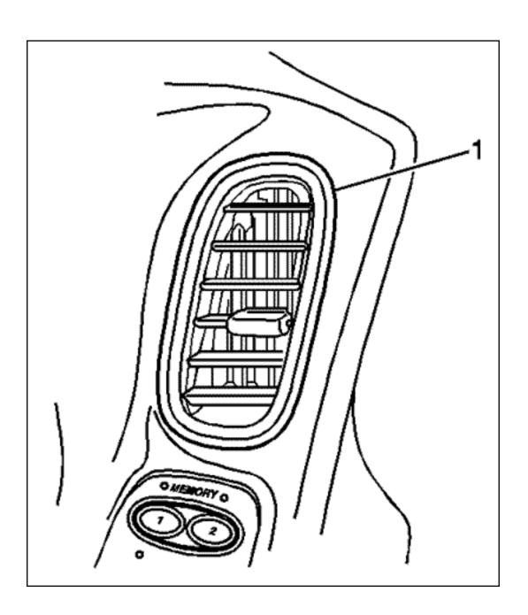
Replace the driver's door HVAC deflector (1), P/N 10406518, if the vanes of the deflector (1) are loose and vibrate. Refer to Door Trim Panel Air Duct and Deflector Replacement in the Service Manual.
