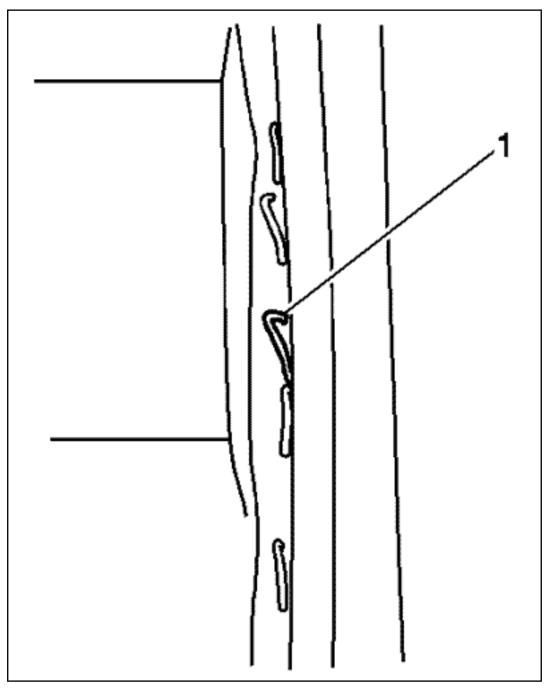
Recrimp or remove any loose staples (1) that retain the door panel leather skin to the door trim panel on the outside perimeter of the door trim panels.
