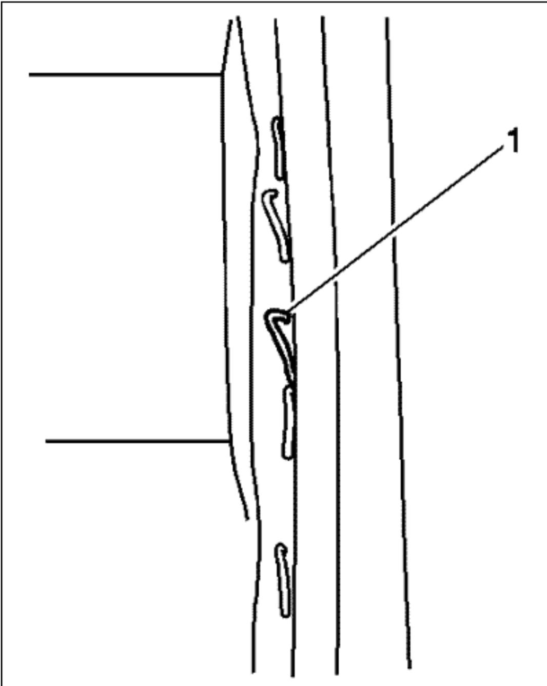
Recrimp or remove any loose staples (1) that retain the door panel leather skin to the door trim panel on the outside perimeter of the door trim panels.
