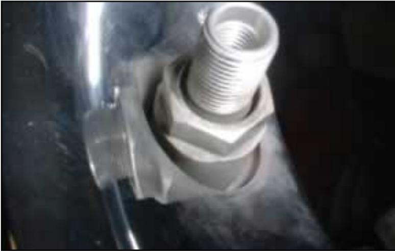
**TIP:** Do not replace either the cap or the valve with standard parts. This will interfere with the sensor's ability to transmit.
