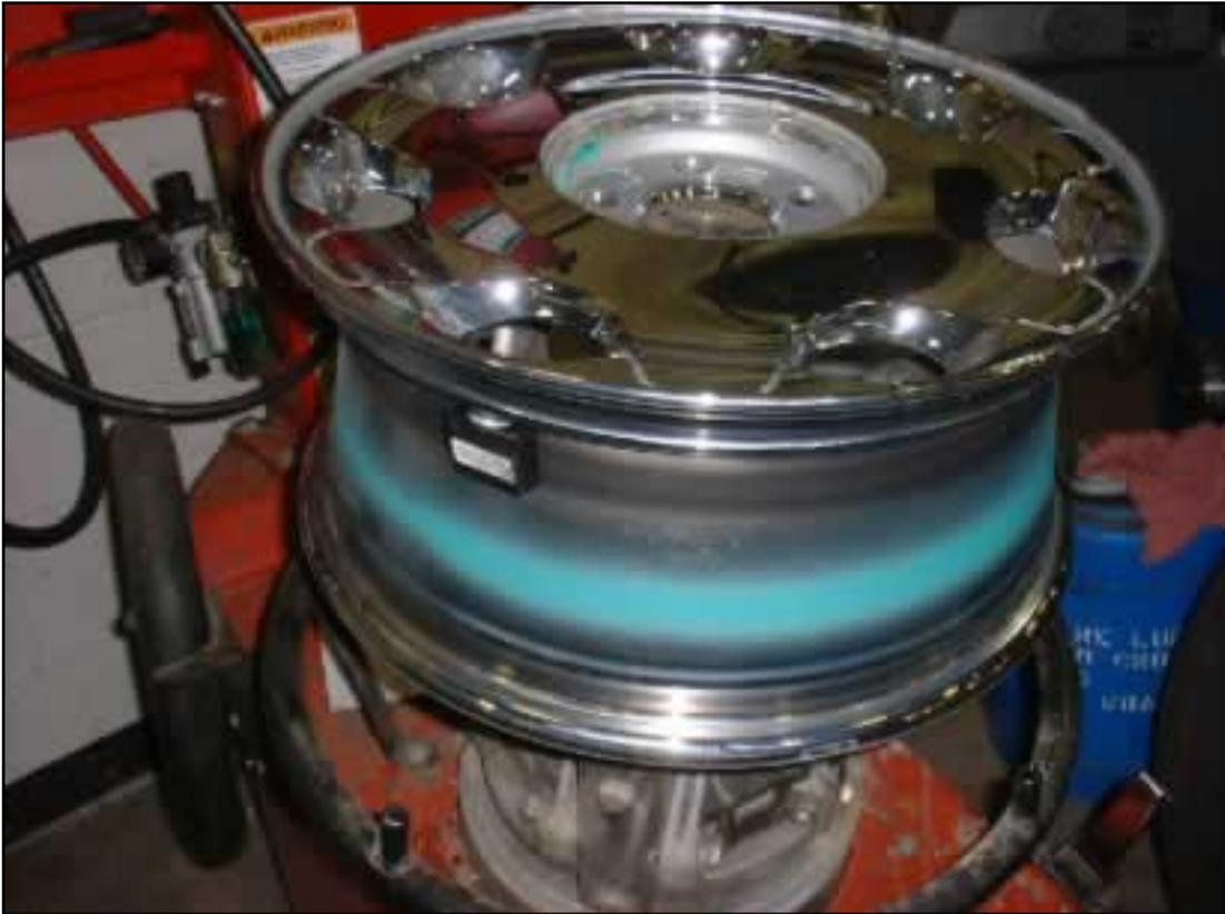
Each sensor is coded differently. This permits the receiver to determine exactly which tire is over or under-inflated.
