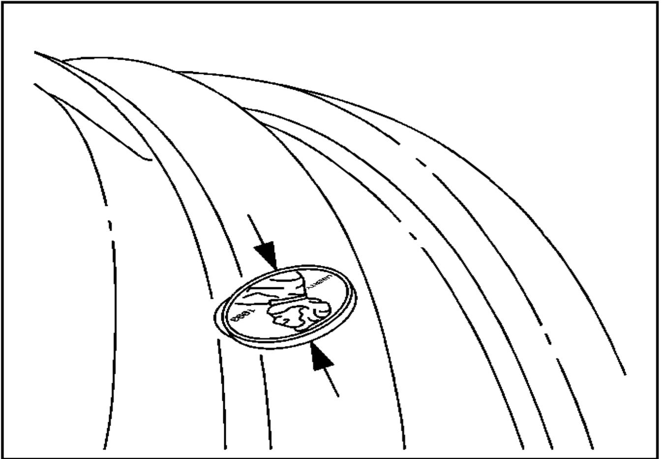
With the tire and valve stem/tire pressure monitor removed from the suspect wheel, place a penny in the counterbore where the valve stem/tire pressure monitor seats on the inside of the wheel. If the penny sits in the counterbore so that it is below the unmachined surface of the wheel at the points indicated by the arrows in the illustration (counterbore depth more than 1.1 mm (.043 in), replace the wheel assembly with the appropriate service part indicated in the chart below.
