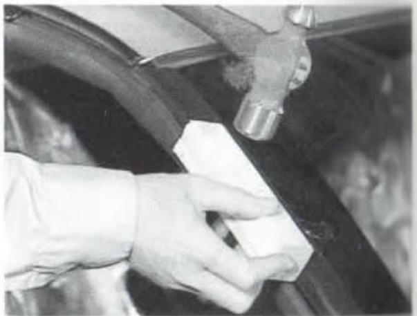
*Bending windshield weatherstrip retainer downward*
