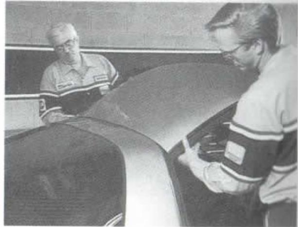
*Pivoting roof panel on dowel pins*
