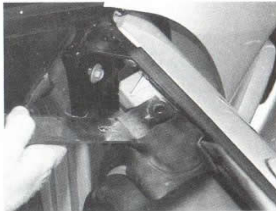
Fir tree fastener at front lip of door weatherstrip
