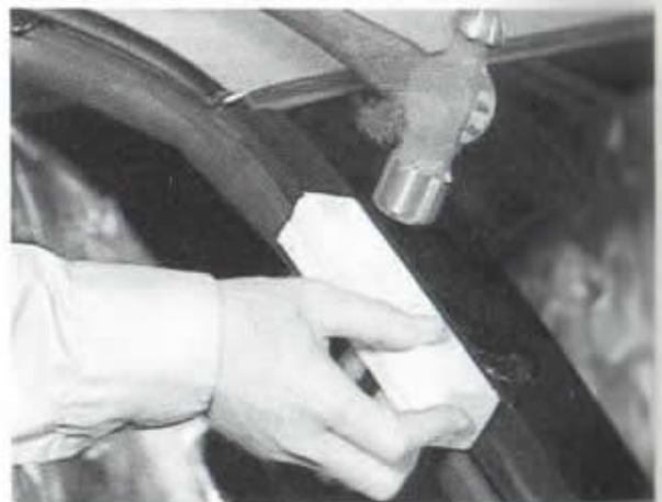
Bending windshield weatherstrip retainer downward
